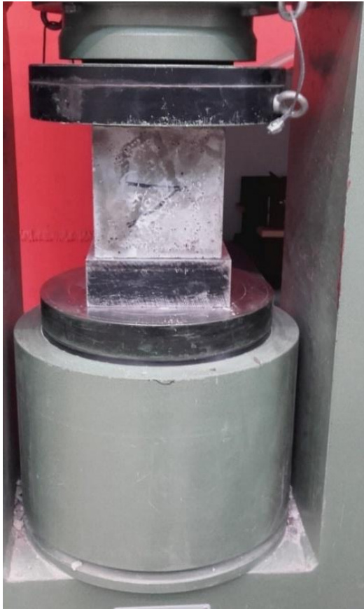
Figur 5.15: Betongkub i betongpress.
