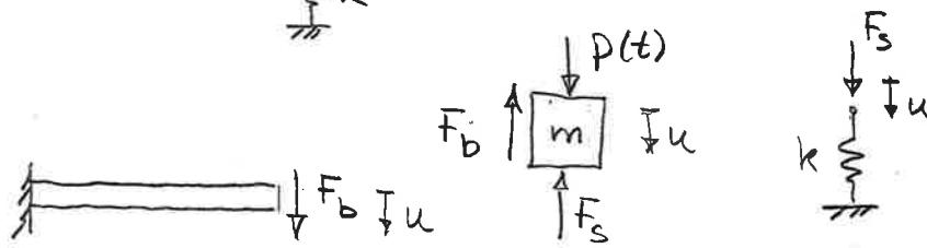
$$\text{Beam: } u = \frac{F_b L^3}{3EI}; \quad F_b = \frac{3EI}{L^3} u \quad \dots (1)$$
