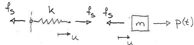
$$\left\{ \begin{array}{l} \text{spring force: } f_s = k u \\ \text{Newton II (mass): } p(t) - f_s = m \ddot{u} \end{array} \right. \dots (1) \quad \dots (2)$$
