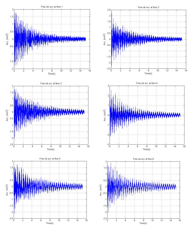
Data in a matrix with eight columns with time first, then the decaying acceleration for floor zero, followed by acceleration for floor one etc. until floor six. The figures above are plots of columns two to eight vs time (the first column). Data is found in a file named: Transdat
