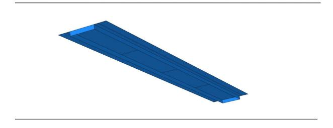
You are provided with a scale model of a bridge-like structure, according to the picture above, for laboratory testing. It is a slender structure, made of steel, sensitive to bending and torsion and it is going to be analysed in terms of its dynamic response. You are to perform laboratory measurements and dynamic FE analyses using ABAQUS on the scale model.
