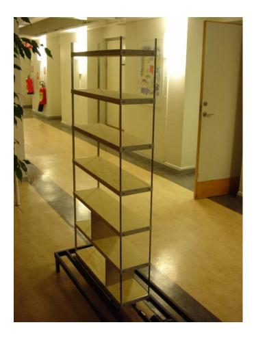
The assignment concerns a six-storey frame (shown in the photo) and its low frequency structural vibrations. It is an idealized scaled model of a so called Shear-building. It consists of 7 wooden plates connected by four steel strips.
