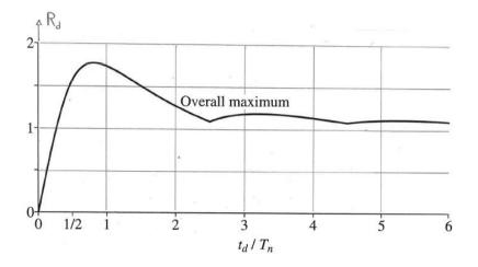
Determine the maximum dynamic deflection  $u_0$  of the system if the pulse duration  $t_d$ =0.2s and the force maximum is  $p_0$ =300N.
