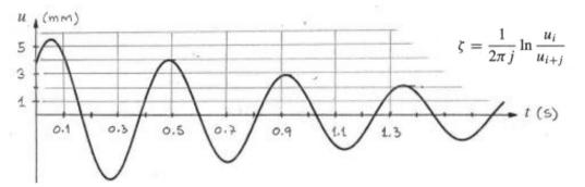
Determine the natural angular frequency  $\omega_n$  and the damping ratio  $\zeta$  of the system. If the mass m=2kg what is then the stiffness of the spring?
