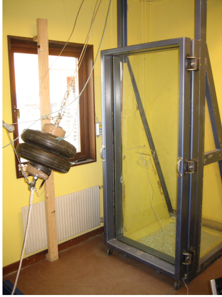
Figure 1: Test arrangement for pendulum impact test.
