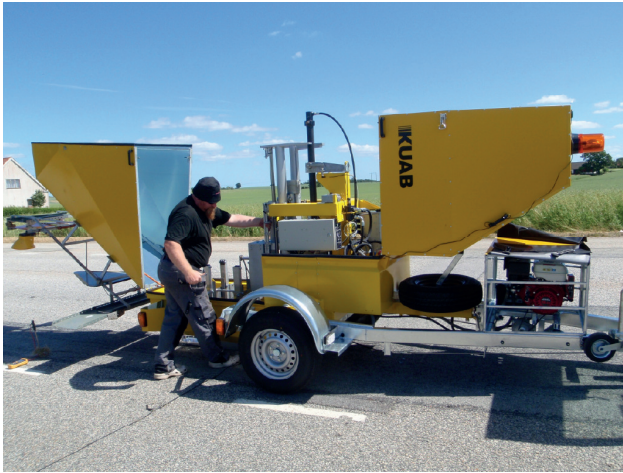
(a) The FWD machine that generates an impulse load.
