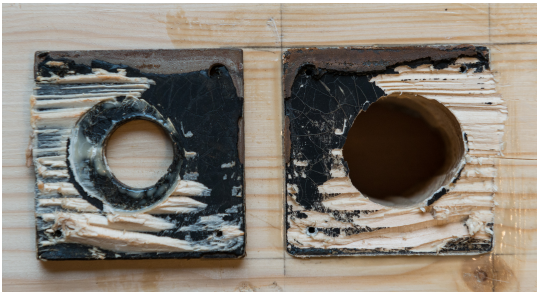
Figure 5: Illustration of different bond line failure modes of the SPDJ. Failure includes shallow wood shear failure (50%), failure in the adhesive layer including the interlayers (30%) and vulcanization failure (20%). Rubber failure of the tensile type seen here occurred during specimen disassembly, after the tests. The steel plate was intentionally mounted eccentric over the over-sized timber hole in order to facilitate a large enough displacement at failure to register the event in the failure detection system. This specific specimen was in group Par-60, see Table 4.
