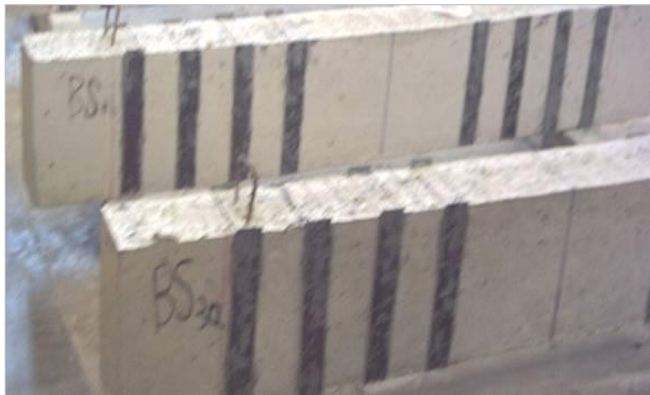
Fig. 10. CFRP laminate in test series RS1.
