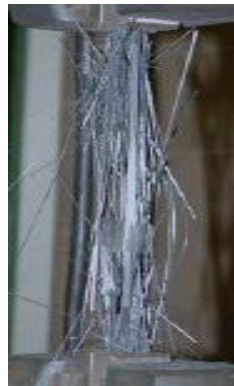
Fig. 3. The failure of a CFRP laminate specimen.
