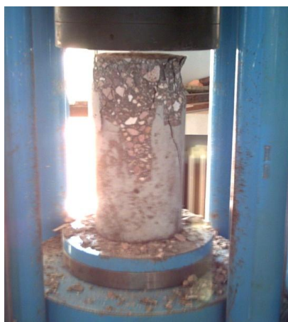
Fig. 1. Concrete specimen in cylinder compression test.
