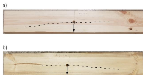
Figure 10: Typical failure modes observed for unmodified (a) and acetylated wood (b).
