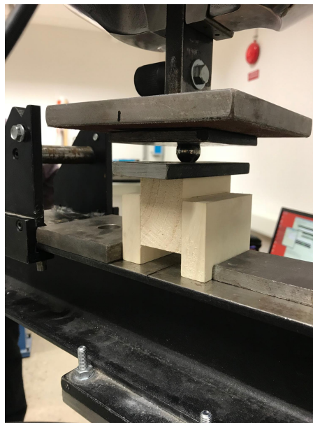
Figure 5.4: Setup in the MTS-Machine.
