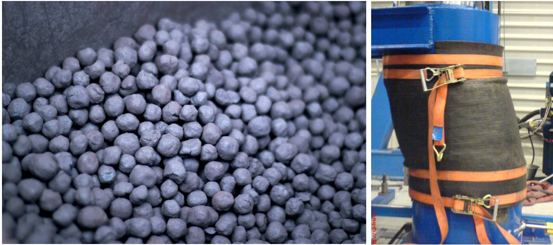
Figure 2.2: Left: A closeup picture of iron ore pellets. Image courtesy LKAB. Right: The arrangement of the rubber cylinder containing iron ore pellets during shear test [6].
