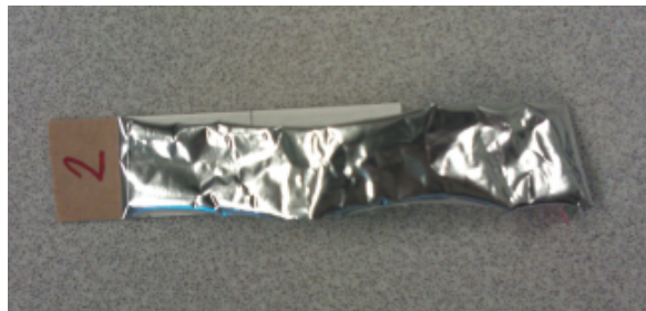
Figure 6.4: Adhesion 2 specimen, separation of the Inside layer and Aluminum layer to the Laminate layer.
