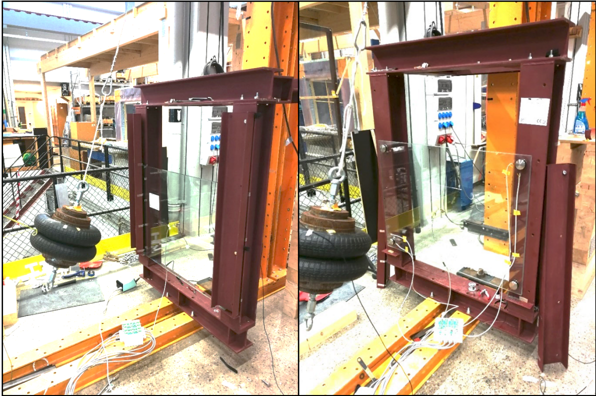
Figure 5-1: Examples of the experimental setup, with simply supported (left) and bolted (right) fastener configurations.
