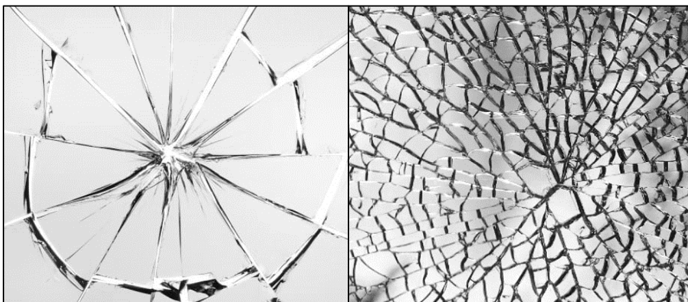
Figure 3-3: Principal breakage patterns of annealed (left) and tempered glass (right). Source: Custom Glass Products, 2020.
