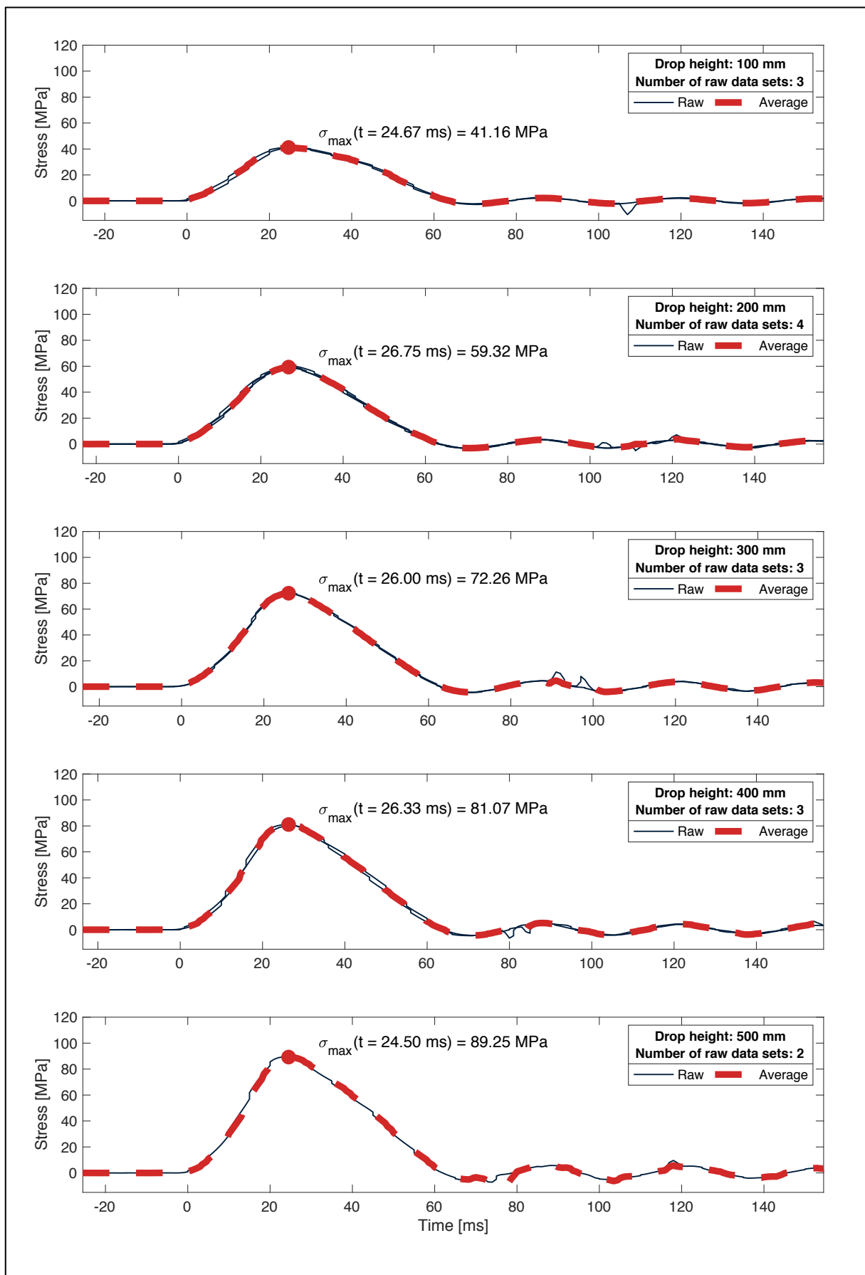
Figure A-10: Principal stress at glass specimen impact location for various impactor drop heights. The data are derived from a strain gauge positioned at the tensile face of the specimens during the experimental campaign. The data set corresponds to clamped laminated specimens with a thickness profile of 6 mm ESG + 1.6 mm SGP + 6 mm ESG.
