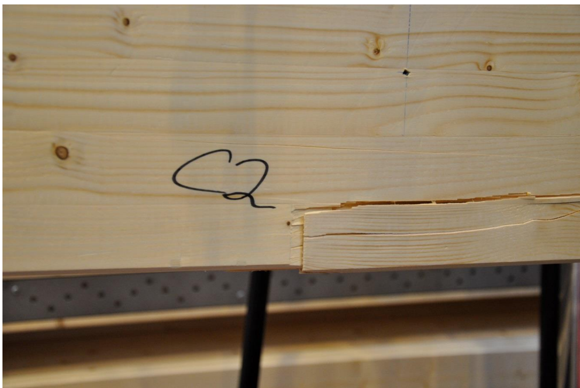
Figur 6.55- Balk C2, dragbrott i fingerskarv.
