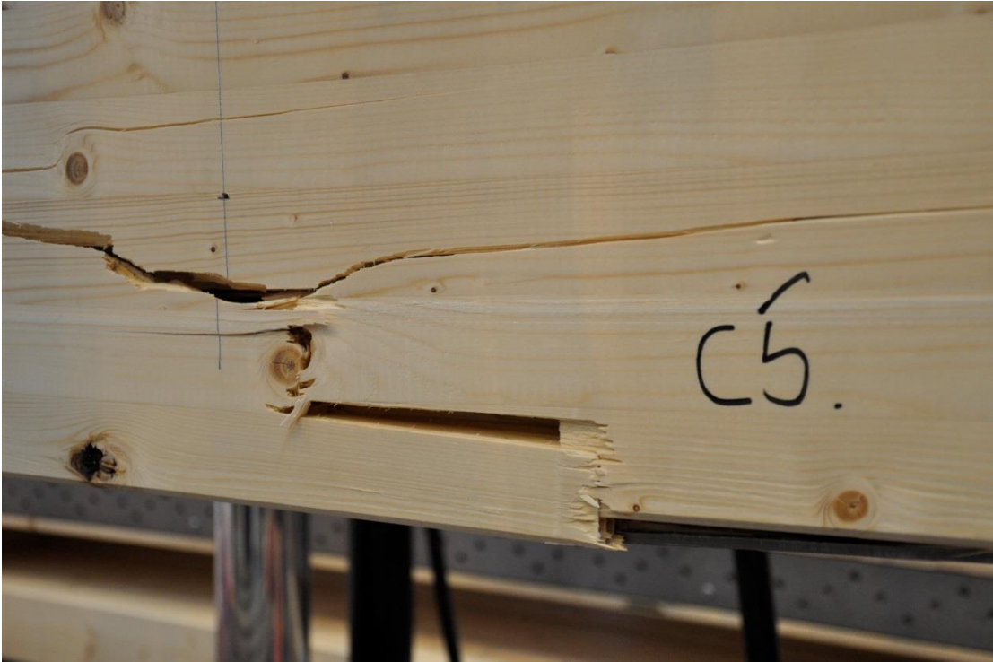
Figur 6.61- Balk C5, dragbrott i fingerskarv.
