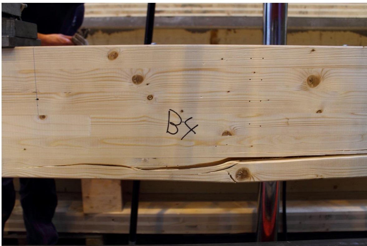
Figur 6.47- Balk B4, dragbrott runt kvist.
