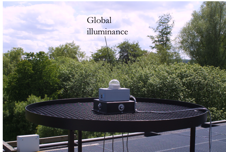
Figure 2.7 Picture showing the lux meter on the roof for recording the global illuminance (photo Jan Carl Westphall).
