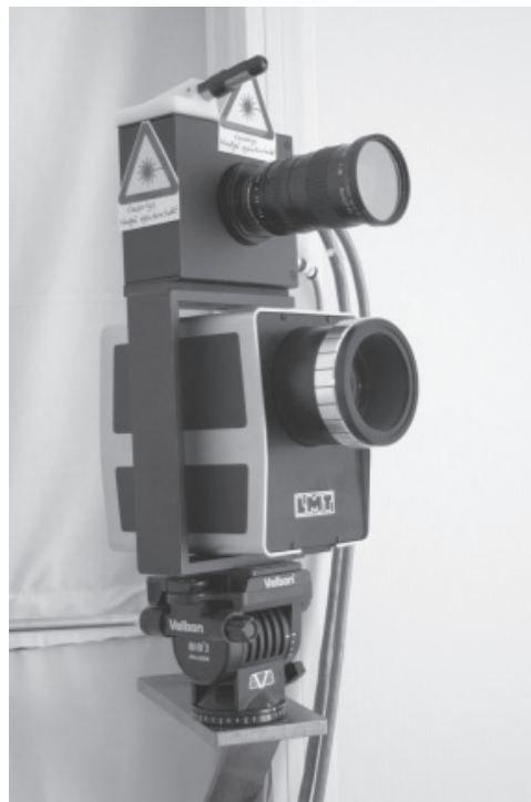
Figure 2.10 Photograph showing the supports for the CCD camera and electronic luminance meter mounted under the camera. The picture also shows the laser beam (top of camera) which was used to adjust the position of the camera (photo Jan Carl Westphall).
