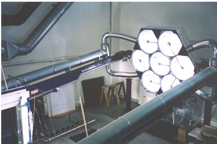
Figur 3.1 Solsimulatorn (A) i LTHs sollaboratorium
