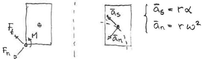
$$(\swarrow) \quad F_n = m \bar{a}_n \quad ; \quad F_n = m r \omega^2 \quad \dots (1)$$
