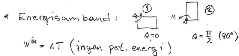
$$W_{ik} = M \cdot \frac{\pi}{2} \quad \text{och} \quad T_1 = 0 \quad \text{och} \quad T_2 = \frac{1}{2} I_0 \omega^2 \Rightarrow$$
