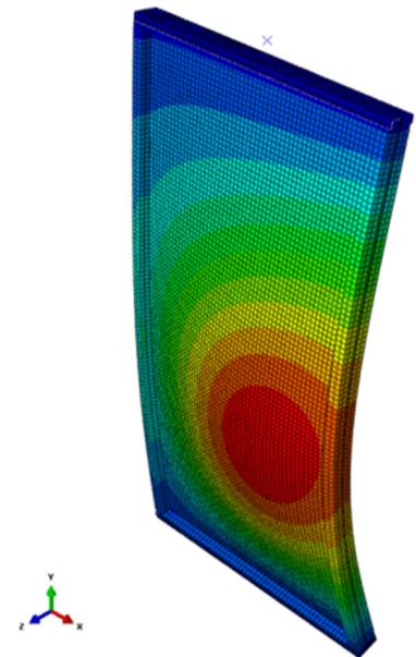
The finite element model will be calibrated to match the results from experiments in terms of failure loads assuming failure is due to instability in the shear wall element.
