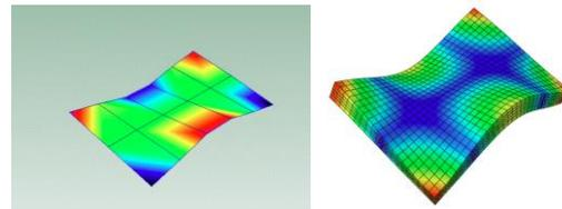
Figure 2. Experimental vibration mode (left) and computer-based vibration mode (right).
