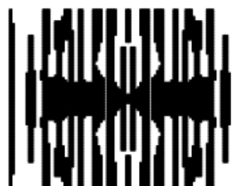
Figure 3: Example of how an optimized configuration of the elastomer layer can appear, seen from above. Black areas are elastomer and white are void.
