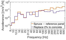
The accelerance response in third octave bands, when replacing 2% of spruce to concrete in comparison to the reference panel.
