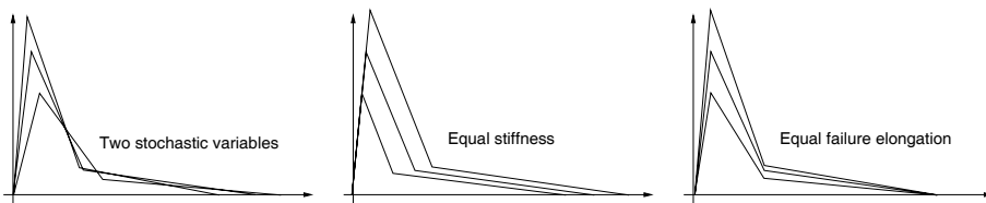
Figure 10: Left: The model with two stochastic variables, Center: Equal stiffness, Right: Equal failure elongation
