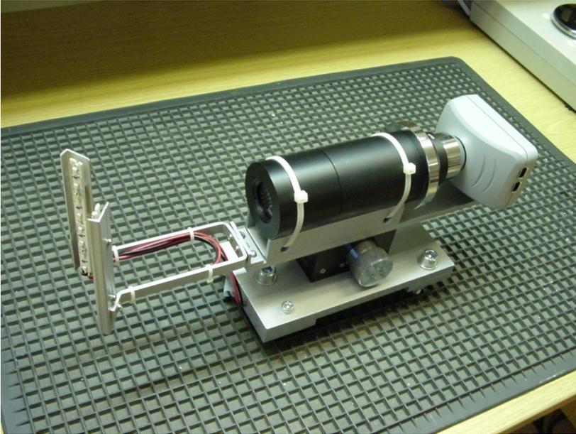
*Figure 1. Digital camera with mounting and light ramp.*
