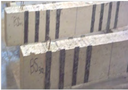
Figure 3. Installation CFRP in experimental work.
