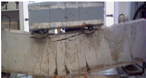
Fig. 12. Flexural failure for control beam.
