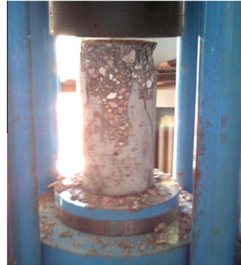
Fig. 1. Concrete specimen in cylinder compression test.
