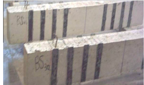
Fig. 10. CFRP laminate in test series RS1.
