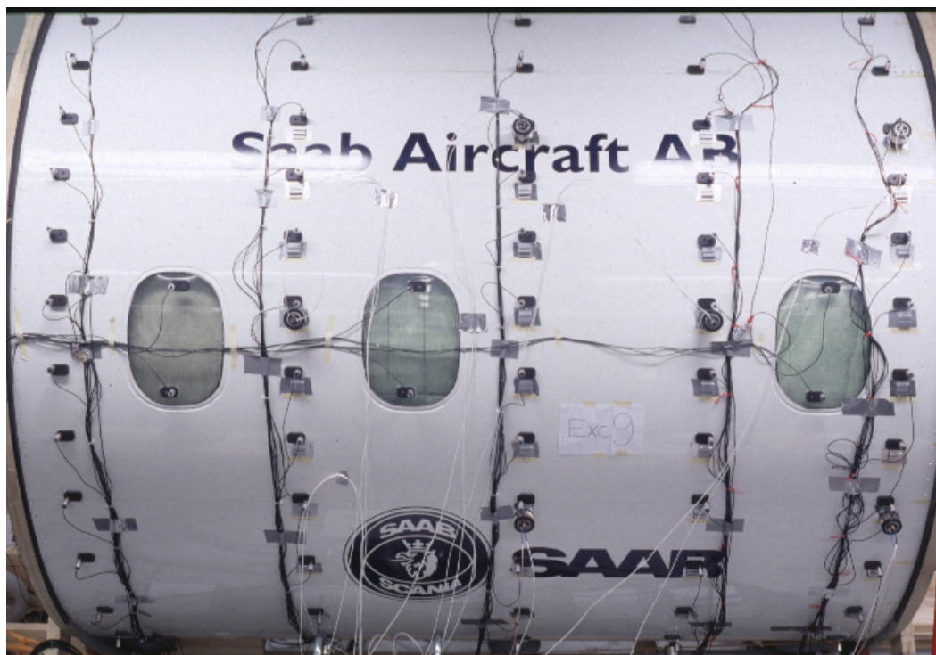
Figure 4: The Saab 340 acoustic test section.
