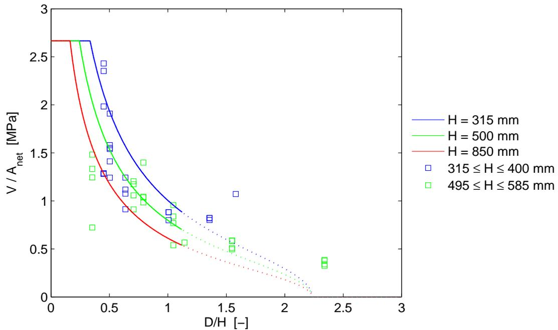
Figure 5.15: Characteristic capacity  $V_k/A_{net}$  according to *Limträhandbok method 2* for different beam heights compared to  $V_c/A_{net}$  for experimental tests on rectangular holes ( $D = \sqrt{a^2 + b^2}$ ).  $V_k/A_{net}$  based on hole side length ratio  $a/b = 2.0$ .
