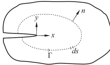
Figure 3.4: *Notations used in J-integral method.*
