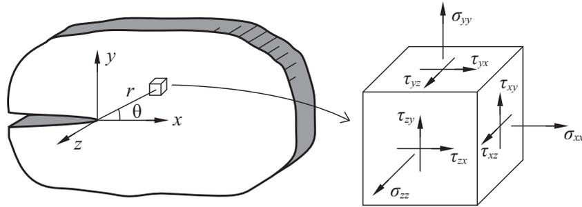
Figure 3.3: *Stresses used in definition of stress intensity factors.*
