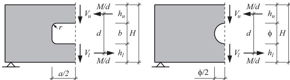
Figure 5.1: Notations for design according Method 1, Swedish Limträhandbok.
