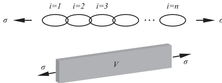
Figure 3.7: Chain consisting of  $n$  discrete links (top) and volume  $V$  consisting of  $V/dV$  unit volumes  $dV$  (bottom).
