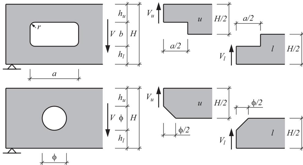
Figure 5.2: Notations for design according Method 2, Swedish *Limträhandbok*.
