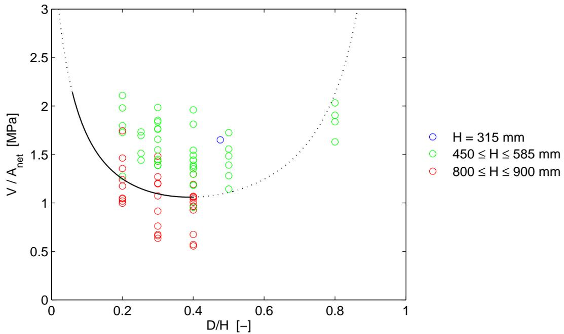
Figure 5.16: Characteristic capacity  $V_k/A_{net}$  according to DIN 1052:2004 compared to  $V_c/A_{net}$  for experimental tests on circular holes ( $D = \phi$ ).  $V_k/A_{net}$  valid for all beam heights  $H$  and based on bending moment to shear force ratio  $M/(VH) = 2.0$ .
