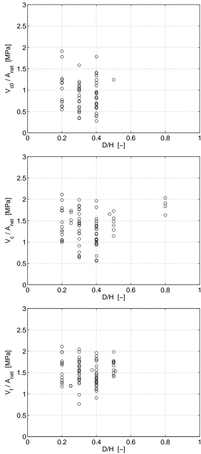
Figure 2.8: Mean shear stress  $V/A_{\text{net}}$  for load levels  $V_{c0}$  (top),  $V_c$  (middle) and  $V_f$  (bottom) for circular holes in shear force dominated region.  $D = \phi$ .
