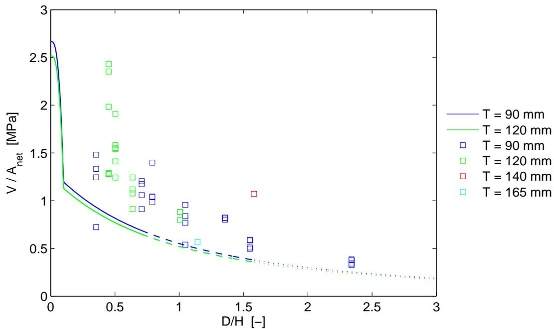
Figure 5.13: Characteristic capacity  $V_k/A_{net}$  according to *Limträhandbok* method 1 for different beam widths  $T$  compared to  $V_c/A_{net}$  for experimental tests on rectangular holes ( $D = \sqrt{a^2 + b^2}$ ).
