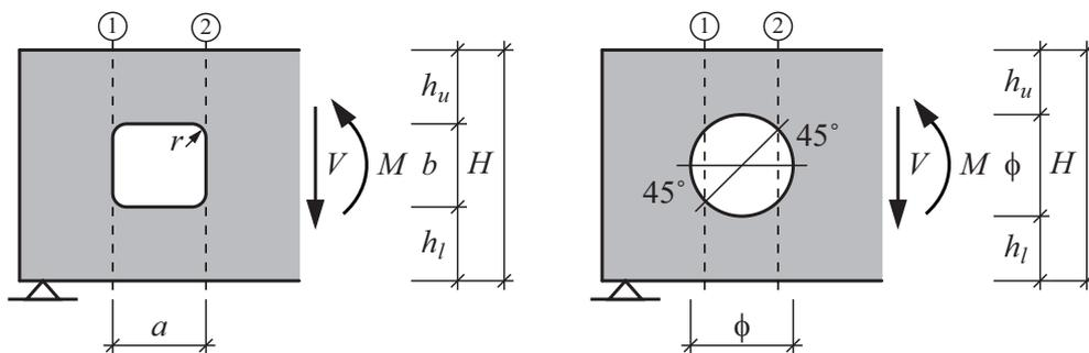
Figure 5.3: Notations for rectangular and circular holes for design according to DIN 1052:2004-08.
