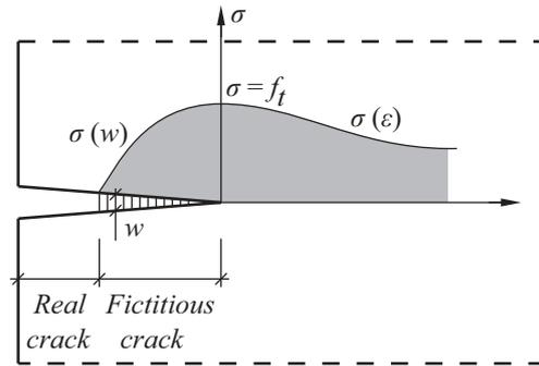
Figure 3.5: *Illustration of stresses in FCM [11].*
