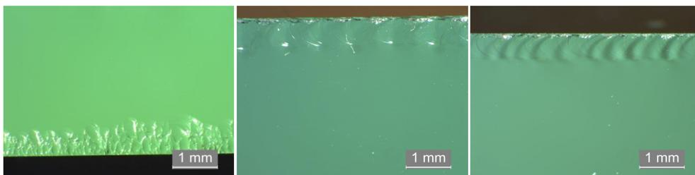
**Figure 2.5:** The cut edge as seen on (left) 4 mm thick glass at opposite side of the scribed edge, (middle) 6 mm thick glass at scribed edge, (right) 8 mm glass at scribed edge. The photographs were acquired with the support of Smart Housing Småland.
