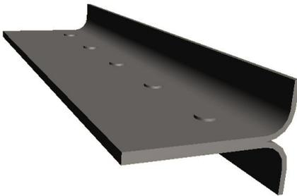
Figure 2.1. T-peel specimen of SPR-joints.
