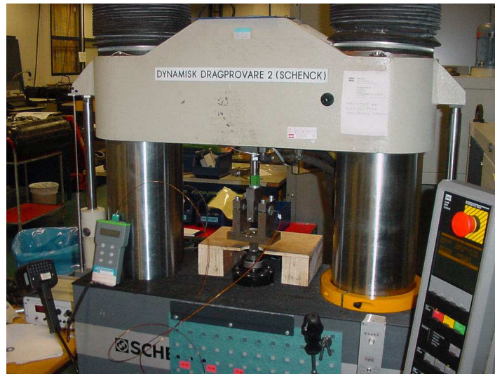
Figure 4.3: The machine used for testing. A Schenck static/dynamic tensile testing machine.
