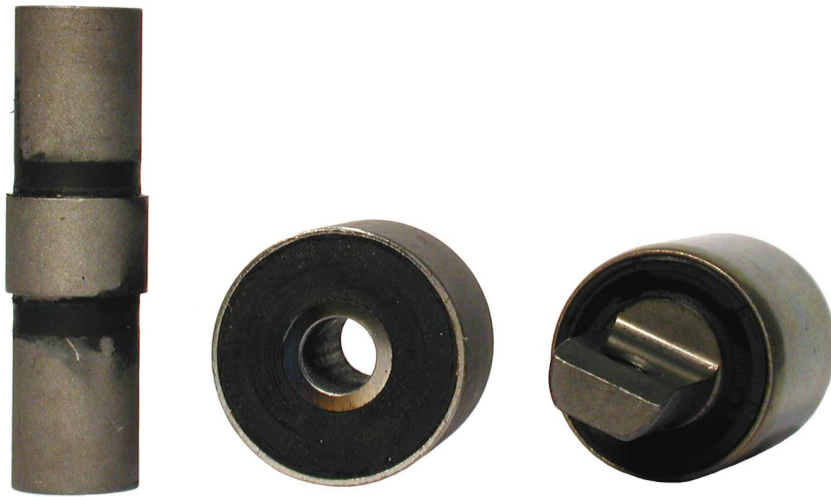
Figure 4.1: The test specimens. From left: shear specimen, cylindrical bushing, and hydrobushing.
