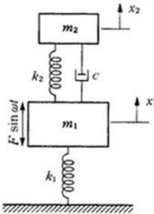
Figure 5.1: TMD attached to an SDF system
