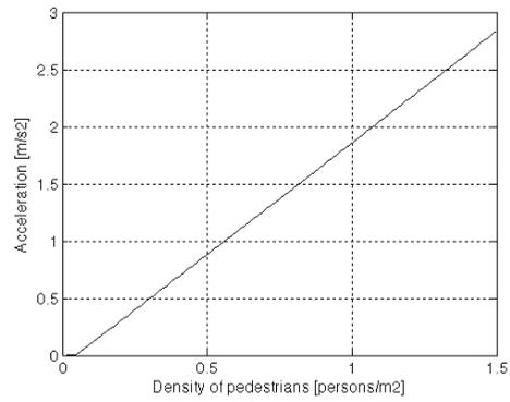
Figure 4.22: Effect of pedestrian density on bridge response
