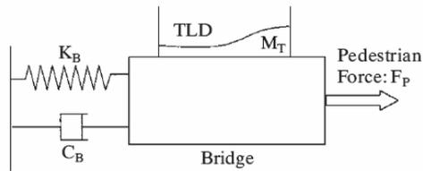
Figure 5.4: TLD attached to an SDOF system [21]
