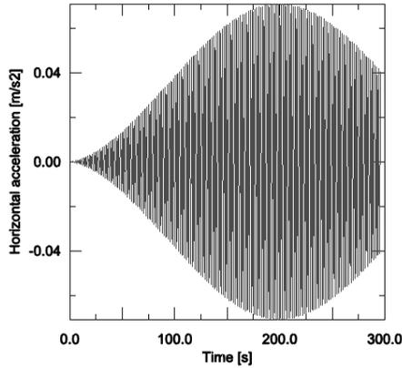
Figure 4.8: Acceleration response, group of non-synchronised people, 1st horizontal natural frequency  $f_1 = 0,517$  Hz
