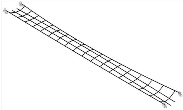
Figure 4.5: Boundary conditions of the FE-model
