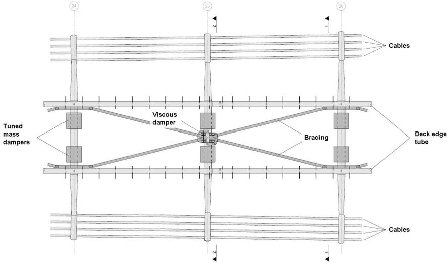
Figure 5.2: Plan of the deck showing placement of TMD and viscous dampers [15]
