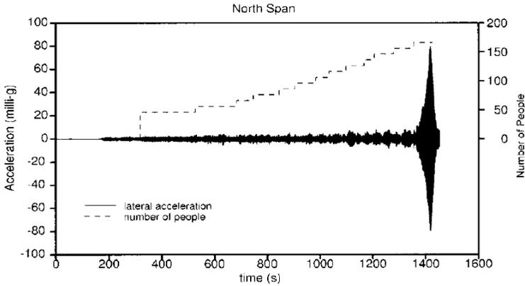
Figure 2.6: Lateral acceleration of the Millennium Bridge and number of pedestrians [8]
