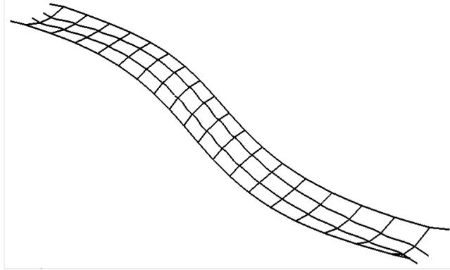
Figure 4.7: 2nd horizontal mode,  $f_2 = 0,971$  Hz
