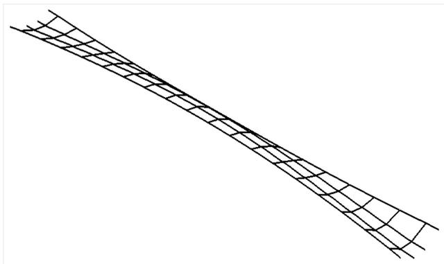
Figure 4.6: 1st horizontal mode,  $f_1 = 0,517$  Hz
