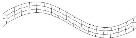
Figure 4.14: The second horizontal modeshape of the Millennium Bridge
