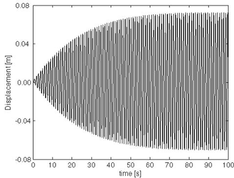
Figure 4.15: Displacement response calculated with the SDOF-model
