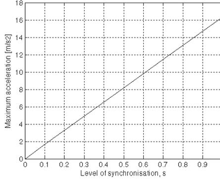
Figure 4.12: Effect of pedestrian synchronisation on bridge response
