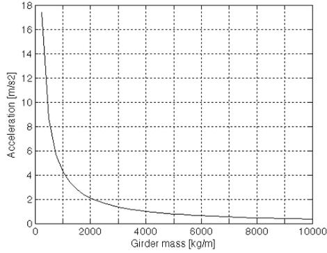
Figure 4.20: Effect of bridge mass on bridge response
