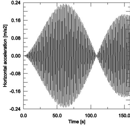
Figure 4.9: Acceleration response, group of fully synchronised people, 2nd horizontal natural frequency  $f_2 = 0,971$  Hz
