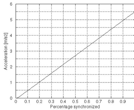
Figure 4.23: Effect of pedestrian synchronisation on bridge response
