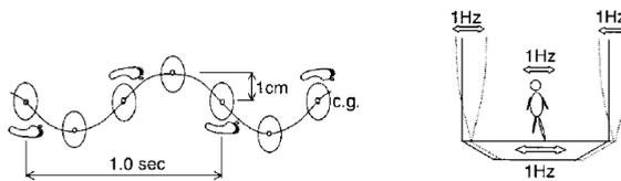
Figure 2.5: Mechanism of lateral vibration [20]
