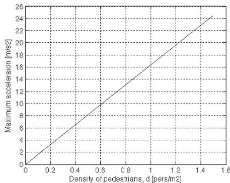
Figure 4.11: Effect of density of pedestrians on bridge response
