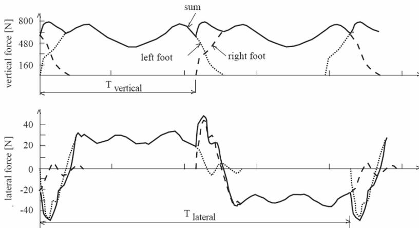
Figure 2.3: Periodic walking time histories in vertical and horizontal directions [38]
