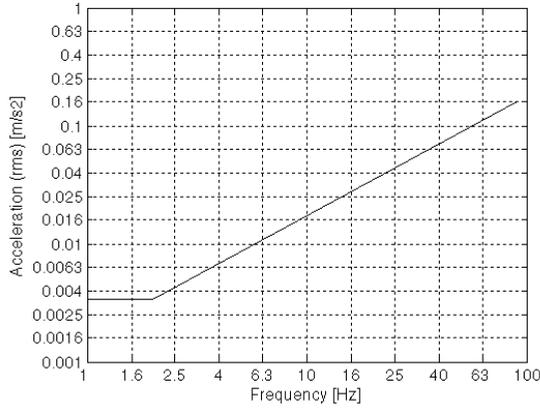
Figure 3.2: Horizontal vibration base curve for acceleration
