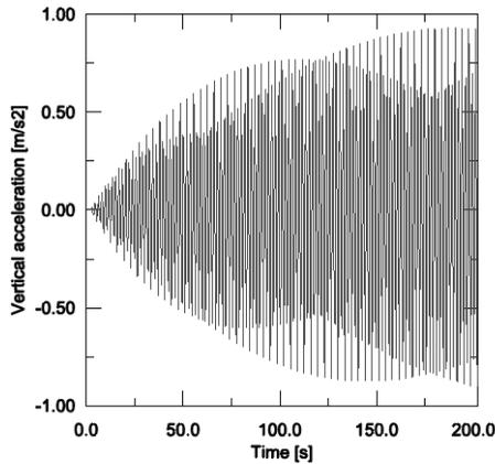
Figure 4.10: Acceleration response, 1st vertical natural frequency  $f_1 = 0,570 \text{ Hz}$
