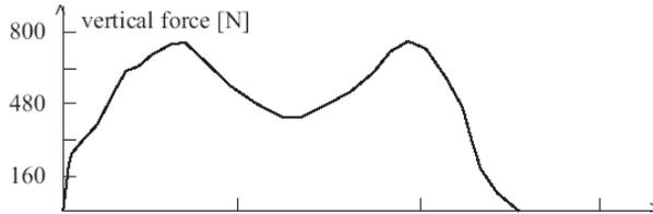
Figure 2.2: Vertical force produced by one person taking one step [38]
