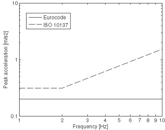
Figure 3.4: Comparison of acceptability of horizontal vibration
