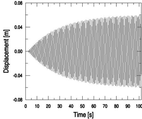
Figure 4.16: Displacement response calculated with the MDOF-model
