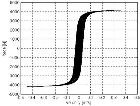
Figure 4.19: Lateral force as a function of bridge velocity
