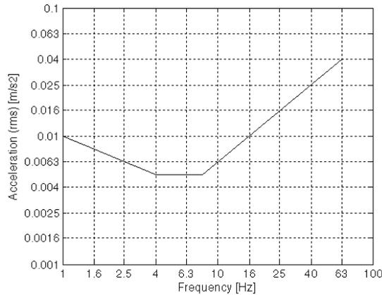
Figure 3.1: Vertical vibration base curve for acceleration
