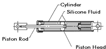
Figure 5.5: Fluid viscous damper [6]
