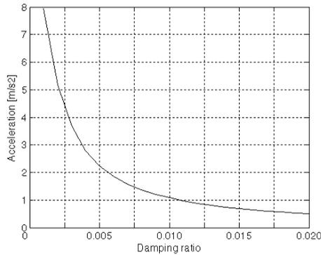
Figure 4.21: Effect of bridge damping on bridge response
