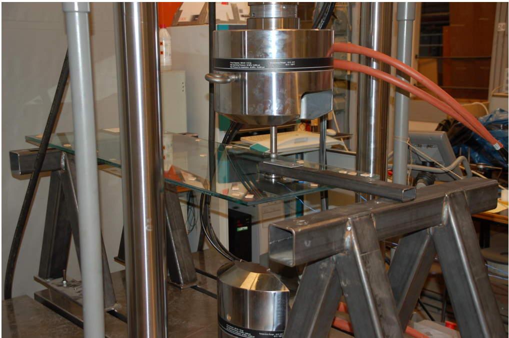
Figure 3-19 MTS machine and the experimental test set-up for the bending test
