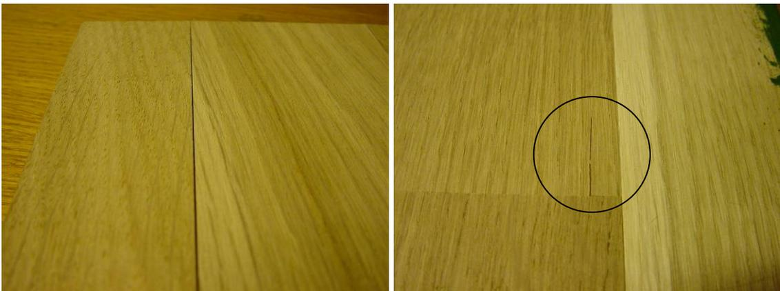
**Figure 3.8:** Left: Failure mode 3, gap opening between oak strip. Right: failure mode 4, crack propagation along fibre direction.
