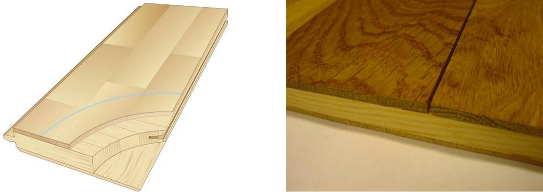
**Figure 1.1:** Left: example of parquet product from Tarkett AB. Right: example of gap opening and delamination of the surface layer.
