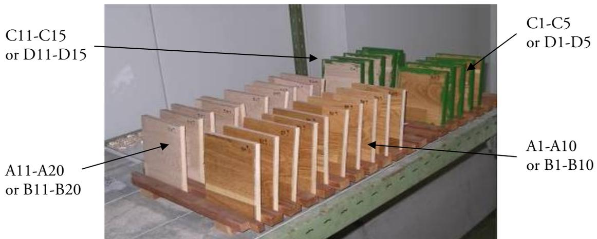
**Figure 3.4:** Different treatment of the surface layer and the edges respectively. Left: specimen without lacquer. Right: lacquered specimens. Front: without edge isolation. Back: isolated edges.
