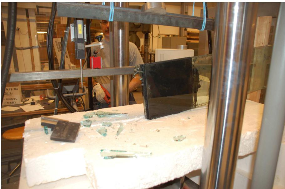
Figure 5.12: *Test set-up of the large-scale test of the adhesive joint Bostik Simson ISR 70-12 after failure in the single flat-glass element.*
