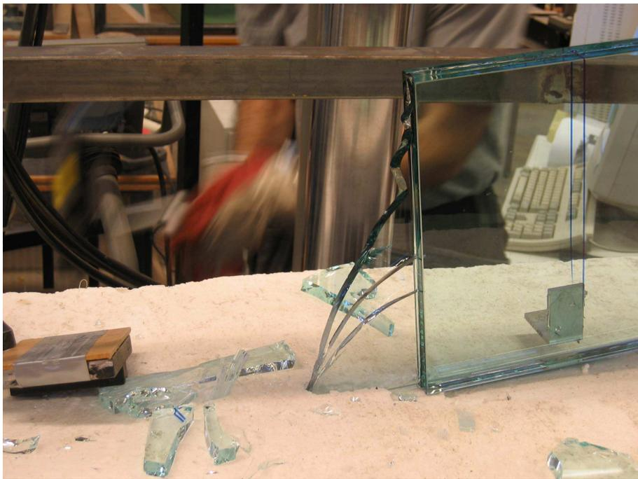
Figure 5.15: *Test set-up of the Casco UV-hardening adhesive joint.*
