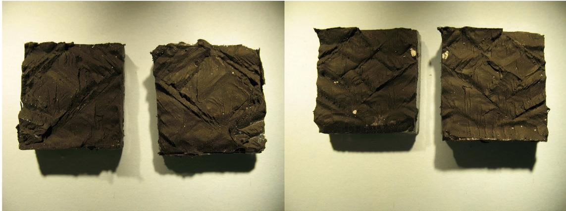
Figure 4.27: *Typical characteristics of the fracture in the specimens of Bostik Simson ISR 70-03.*
