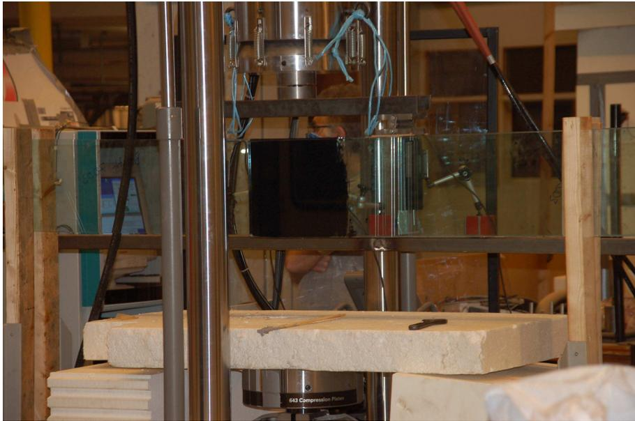
Figure 5.11: *Test set-up of the large-scale test of the adhesive joint Bostik Simson ISR 70-03.*
