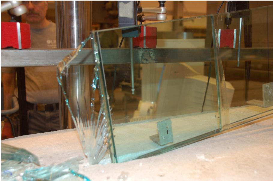
Figure 5.13: *The adhesive joint Casco Strong Epoxy Professional after failure in the single flat-glass element.*
