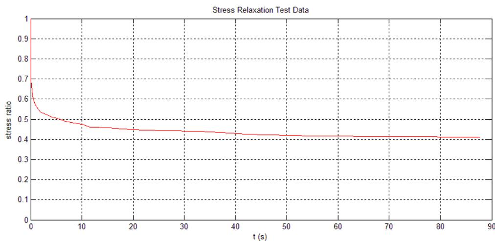
**Figure 4.7.** Stress relaxation test data for PTFE.
