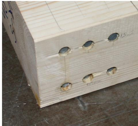
Figure 5.1: The threaded steel screws were irregularly pushed in [5].
