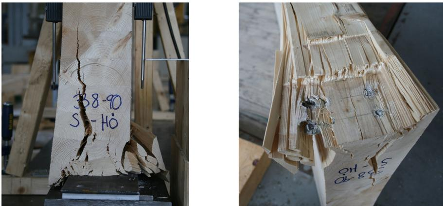
Figure 5.4: To the left, a reinforced beam with threaded steel rods cracks. To the right, a view from the bottom side of the beam [5].
