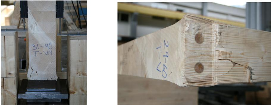
Figure 5.3: To the left, a reinforced beam with dowels cracks both at the right and left side of the beam. To the right, a view from the bottom side of the beam [5].
