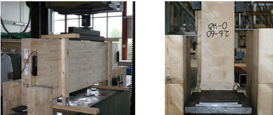
Figure 5.2: To the left, the setup and to the right, a unreinforced beam cracks at the bottom right side of the beam [5].
