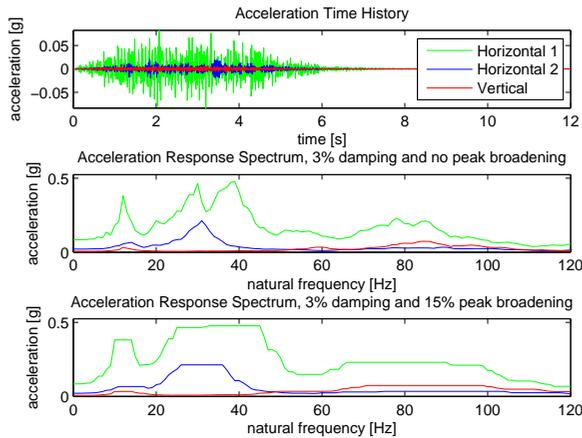
Figure A.13: Three acceleration diagrams for the three principle axis belonging to support B1. First the acceleration time history, then response spectra with no peak broadening and finally response spectra with 15% peak broadening
