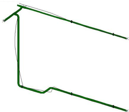
Figure A.24: Fifth eigenmode at 9.14 Hz for the Pipestress Pipe Model
