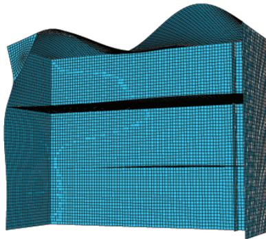
Figure A.10: Ninth eigenmode at 26.42 Hz for the Abaqus Building Model
