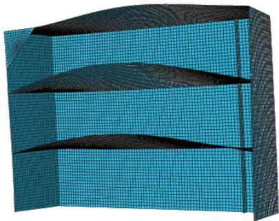
Figure A.5: Fourth eigenmode at 12.55 Hz for the Abaqus Building Model
