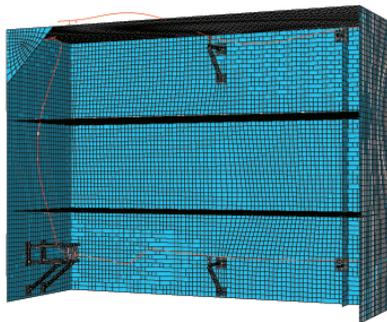
Figure A.31: Fourth eigenmode at 8.87 Hz for the Abaqus Building, Support & Pipe Model
