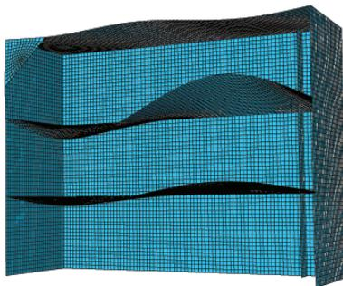
Figure A.8: Seventh eigenmode at 24.72 Hz for the Abaqus Building Model
