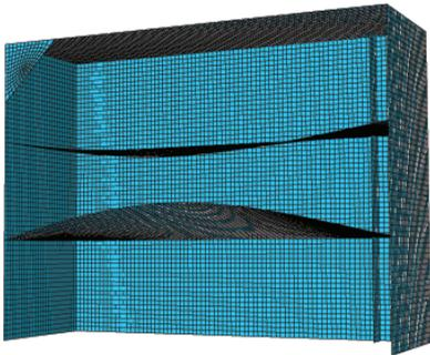
Figure A.4: Third eigenmode at 10.19 Hz for the Abaqus Building Model
