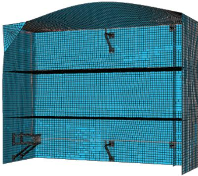
Figure A.29: Second eigenmode at 6.82 Hz for the Abaqus Building, Support & Pipe Model
