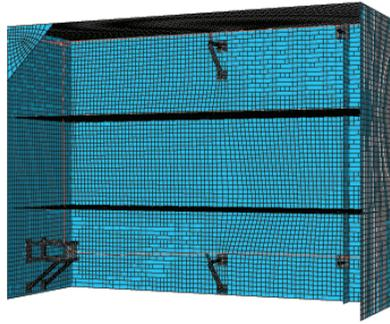
Figure A.33: Sixth eigenmode at 10.00 Hz for the Abaqus Building, Support & Pipe Model
