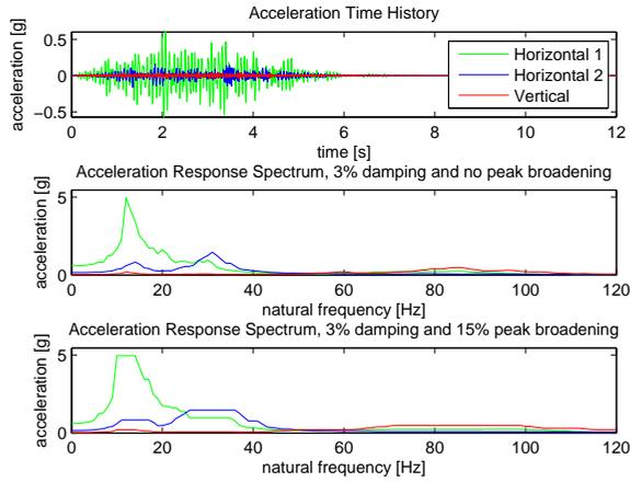
Figure A.16: Three acceleration diagrams for the three principle axis belonging to support B2. First the acceleration time history, then response spectra with no peak broadening and finally response spectra with 15% peak broadening
