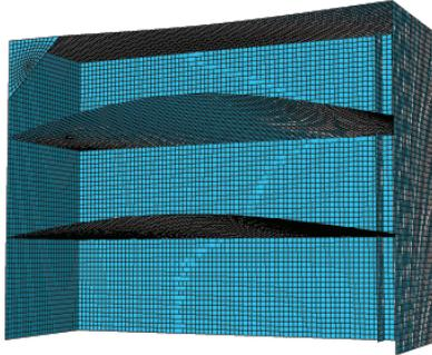
Figure A.3: Second eigenmode at 9.84 Hz for the Abaqus Building Model
