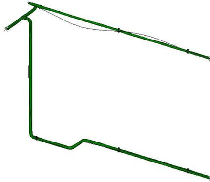
Figure A.26: Seventh eigenmode at 10.57 Hz for the Pipestress Pipe Model
