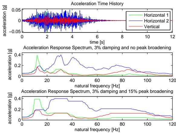
Figure A.14: Three acceleration diagrams for the three principle axis belonging to support C1. First the acceleration time history, then response spectra with no peak broadening and finally response spectra with 15% peak broadening
