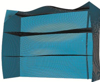
Figure A.11: Tenth eigenmode at 30.55 Hz for the Abaqus Building Model
