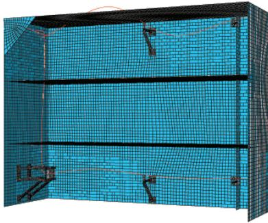
Figure A.35: Eighth eigenmode at 11.46 Hz for the Abaqus Building, Support & Pipe Model
