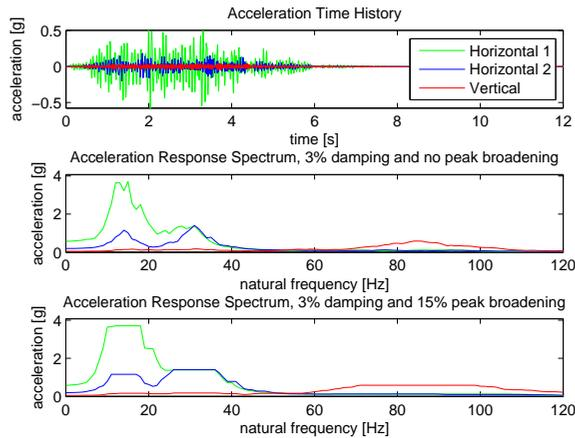
Figure A.15: Three acceleration diagrams for the three principle axis belonging to support A2. First the acceleration time history, then response spectra with no peak broadening and finally response spectra with 15% peak broadening
