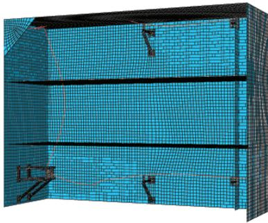
Figure A.30: Third eigenmode at 7.13 Hz for the Abaqus Building, Support & Pipe Model
