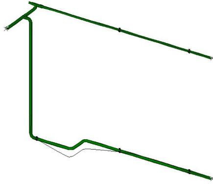
Figure A.22: Third eigenmode at 7.06 Hz for the Pipestress Pipe Model
