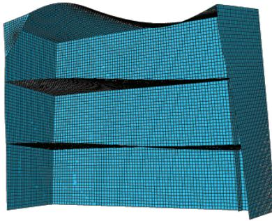
Figure A.6: Fifth eigenmode at 13.77 Hz for the Abaqus Building Model
