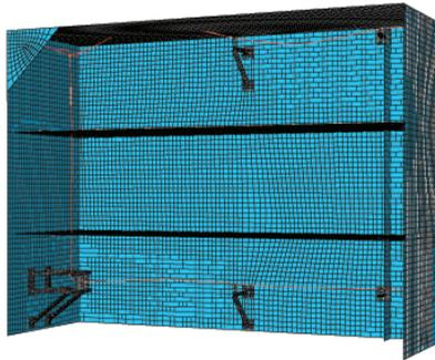
Figure A.36: Ninth eigenmode at 11.65 Hz for the Abaqus Building, Support & Pipe Model
