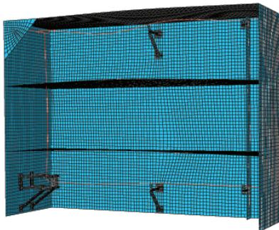
Figure A.37: Tenth eigenmode at 12.51 Hz for the Abaqus Building, Support & Pipe Model
