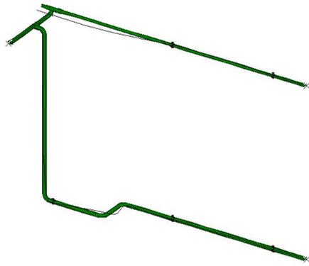
Figure A.23: Fourth eigenmode at 7.38 Hz for the Pipestress Pipe Model
