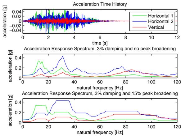
Figure A.17: Three acceleration diagrams for the three principle axis belonging to FIX1. First the acceleration time history, then response spectra with no peak broadening and finally response spectra with 15% peak broadening
