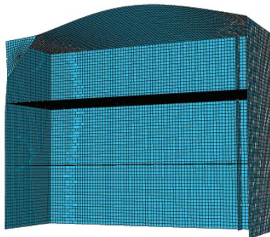
Figure A.2: First eigenmode at 6.83 Hz for the Abaqus Building Model
