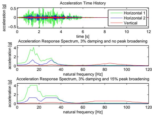
Figure A.18: Three acceleration diagrams for the three principle axis belonging to FIX2. First the acceleration time history, then response spectra with no peak broadening and finally response spectra with 15% peak broadening
