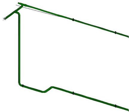
Figure A.21: Second eigenmode at 6.39 Hz for the Pipestress Pipe Model
