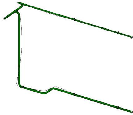
Figure A.25: Sixth eigenmode at 10.00 Hz for the Pipestress Pipe Model
