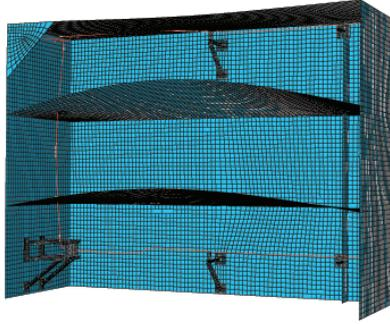
Figure A.32: Fifth eigenmode at 9.84 Hz for the Abaqus Building, Support & Pipe Model
