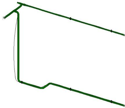
Figure A.20: First eigenmode at 5.34 Hz for the Pipestress Pipe Model
