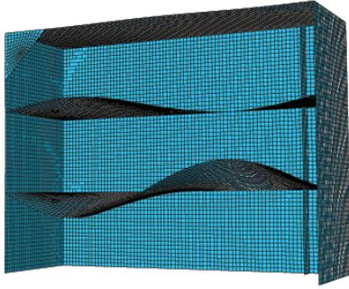
Figure A.9: Eighth eigenmode at 25.08 Hz for the Abaqus Building Model
