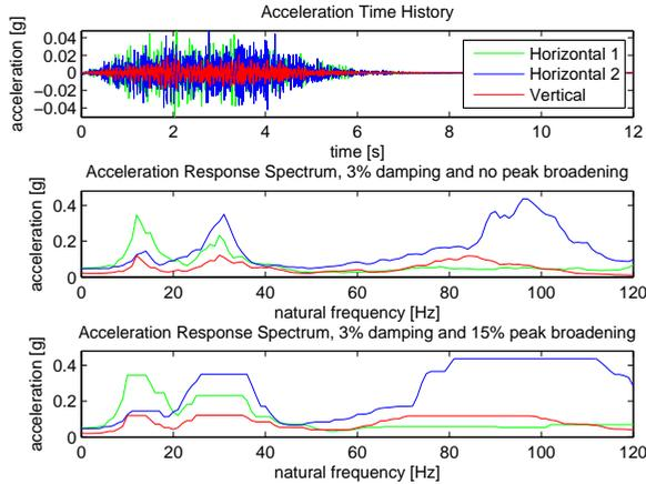
Figure A.12: Three acceleration diagrams for the three principle axis belonging to support A1. First the acceleration time history, then response spectra with no peak broadening and finally response spectra with 15% peak broadening
