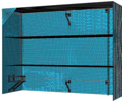
Figure A.27: Abaqus Building, Support & Pipe Model
