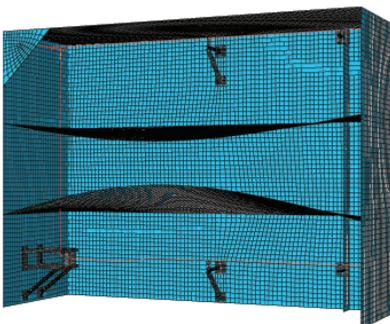
Figure A.34: Seventh eigenmode at 10.17 Hz for the Abaqus Building, Support & Pipe Model
