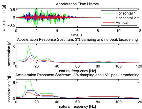
Figure A.19: Three acceleration diagrams for the three principle axis belonging to FIX3. First the acceleration time history, then response spectra with no peak broadening and finally response spectra with 15% peak broadening
