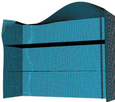
Figure A.7: Sixth eigenmode at 15.63 Hz for the Abaqus Building Model
