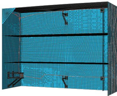
Figure A.28: First eigenmode at 6.57 Hz for the Abaqus Building, Support & Pipe Model
