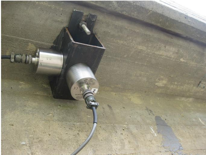
Figure 3.3: Attachment of accelerometers at the roof position
