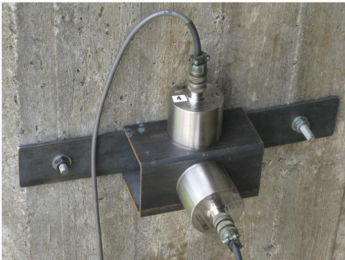
Figure 3.4: Attachment of accelerometers at the wall position
