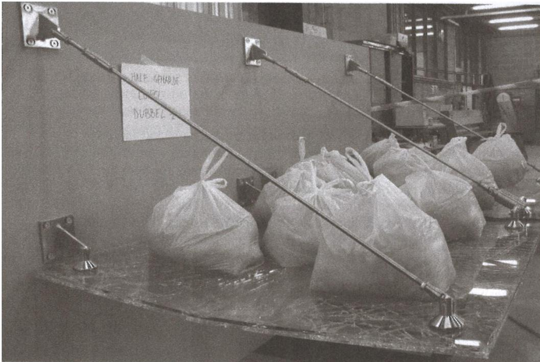
Figure 6.7: Loading of cracked glass plate. Testing carried out by [3].
