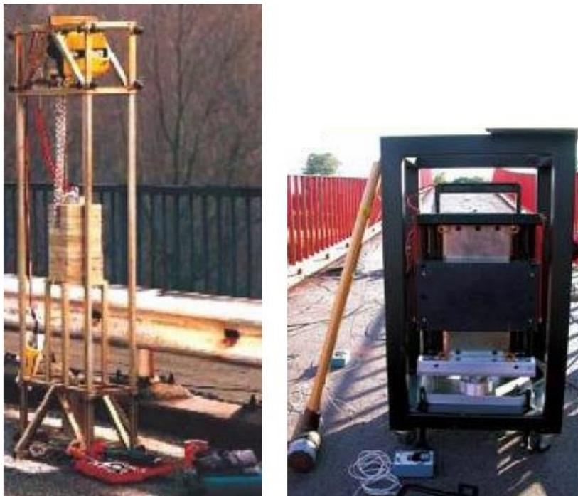
Figure 4.2: Impulse device (left) and electrodynamic shaker and impact hammer (right) [15].
