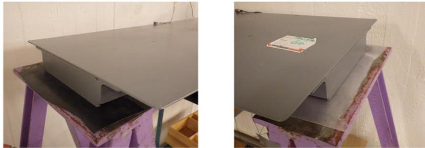
Figure 6.7: Rubber (pinned support) and plastic (roller support) boundary.
