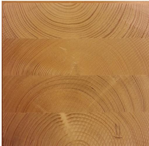
Figure 2.2: Cross- section of glulam. Four Lamellae
