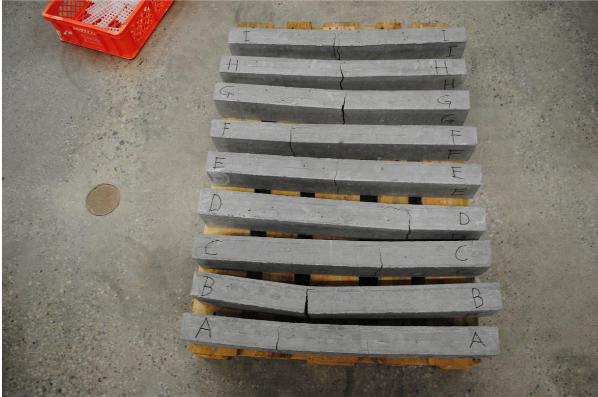
Figure 4.14: Bending cracks of the nine beam specimen.
