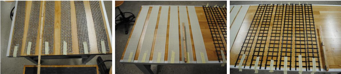
Figure 4.6: The reinforcement specimen: steel, glass and carbon fabrics. From the left-hand side steel, glass and carbon.
