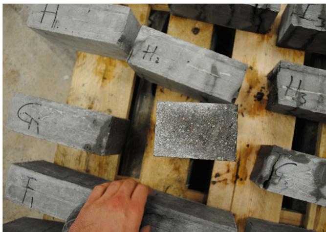
Figure 4.13: Section cut of a carbon reinforced beam (beam G).
