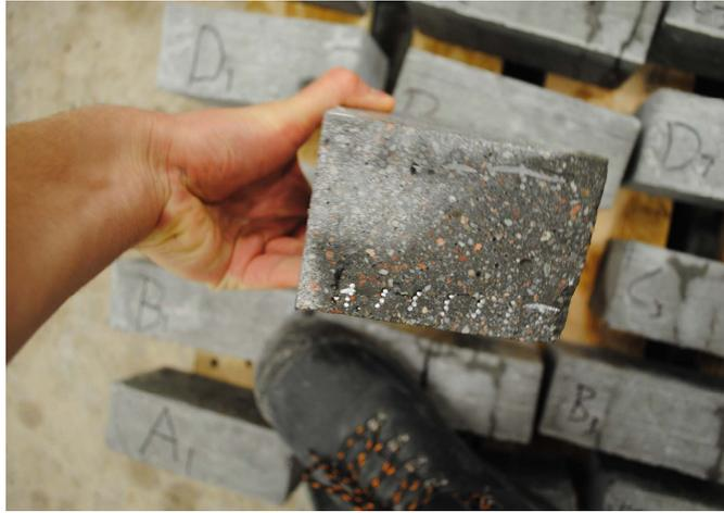
Figure 4.11: Section cut of a steel reinforced beam (beam C).
