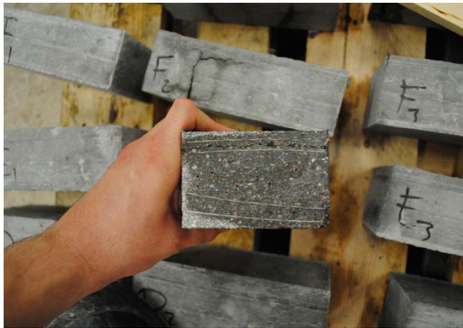
Figure 4.12: Section cut of a glass reinforced beam (beam E).
