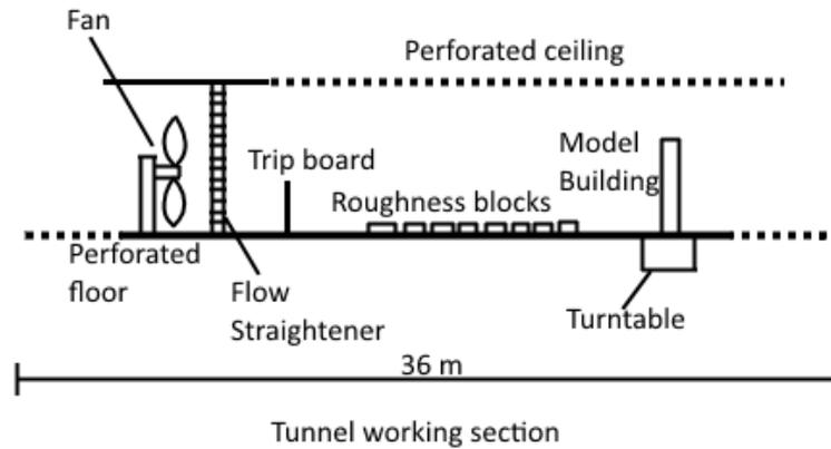
Figure 3.15: Illustration of wind tunnel tests [64].
