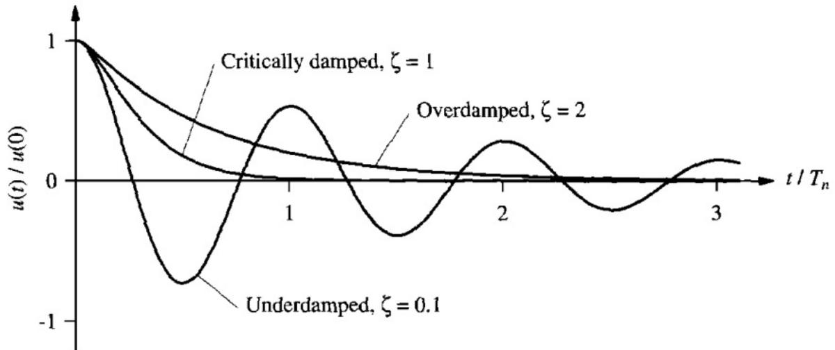
Figure 3.11: Free vibration of underdamped, critically damped and overdamped systems [10].
