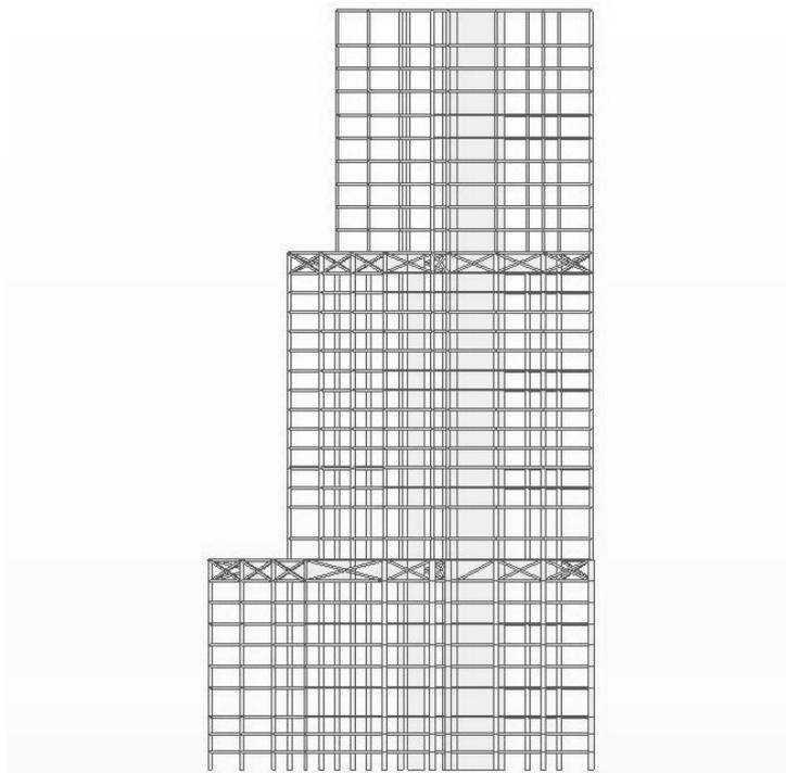
Figure 5.28: Outrigger placed on two floors.
