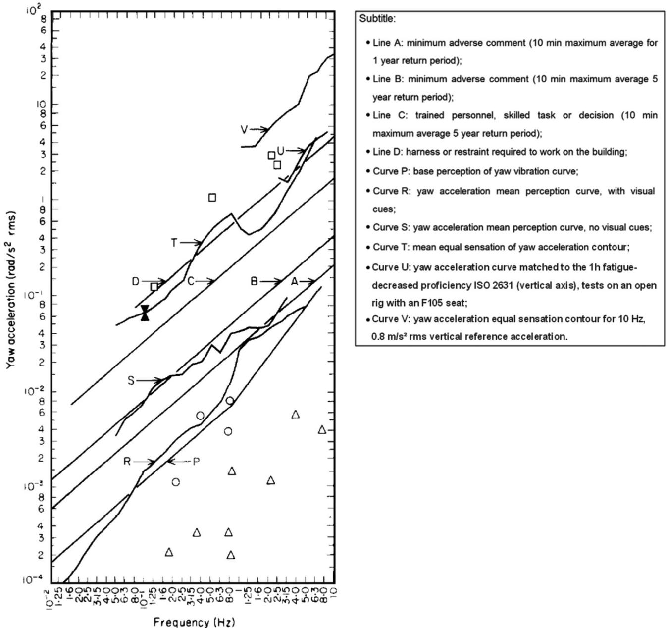
Figure 3.2: Human response and recommendations to yaw acceleration [37].
