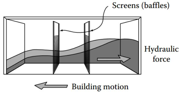
Figure 3.12: Tuned sloshing damper [64].
