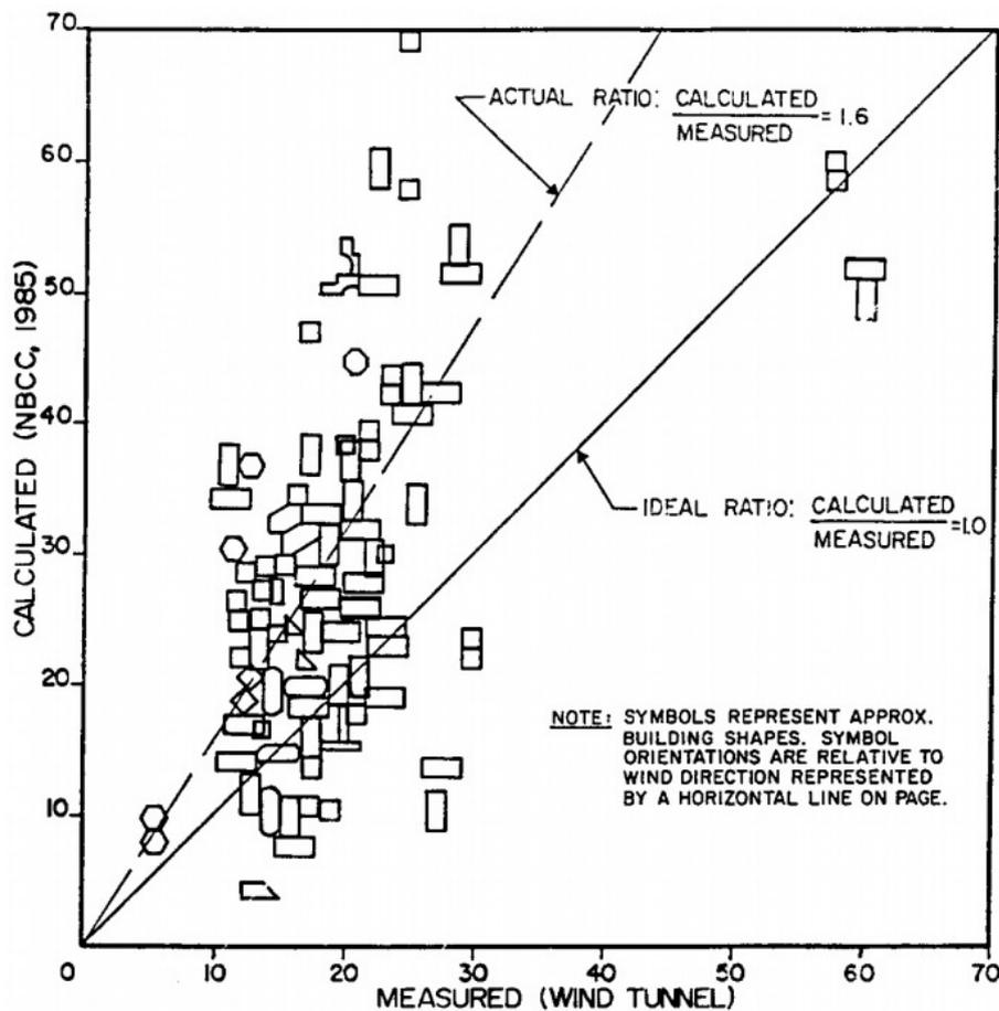
Figure 6.3: Calculated accelerations according to NBCC compared to results from wind tunnel tests [22].
