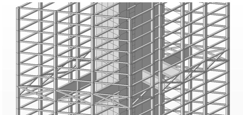
Figure 5.27: Illustration of outrigger.
