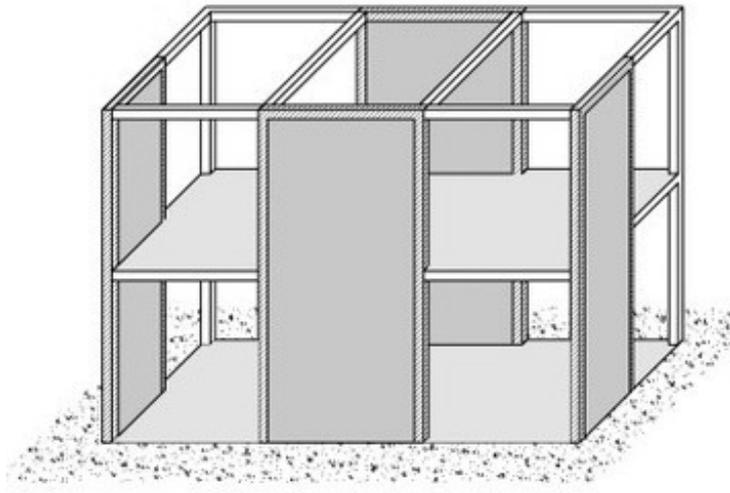
Figure 2.3: Illustration of shear walls [25].
