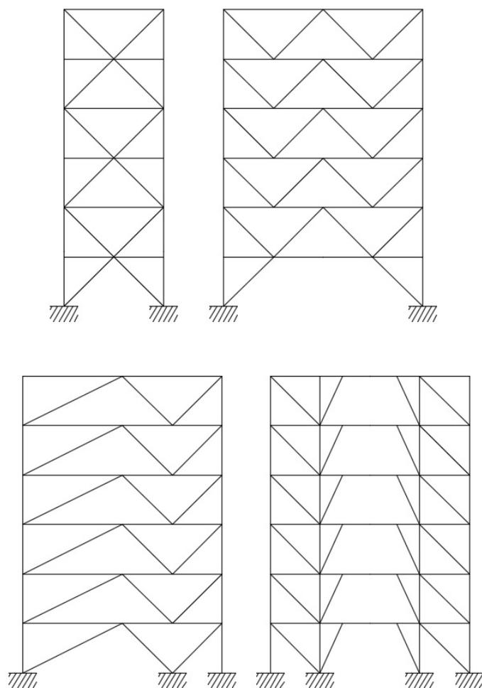
Figure 2.6: Illustration of concentric braced frames [64].
