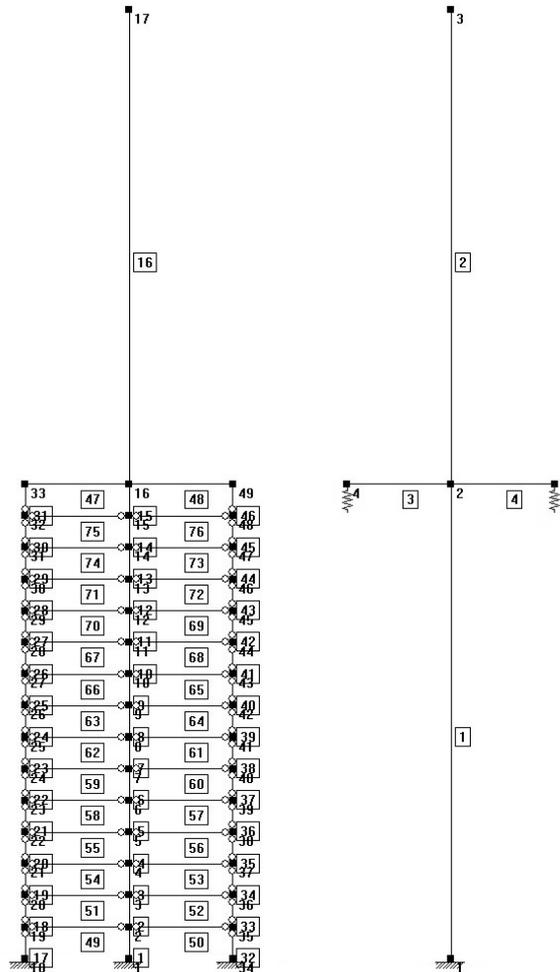
Figure 5.24: Illustration of the two Strusoft Frame Analysis models, model 1 on the left and model 2 on the right.
