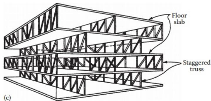
Figure 2.8: Illustration of a staggered truss system [64].
