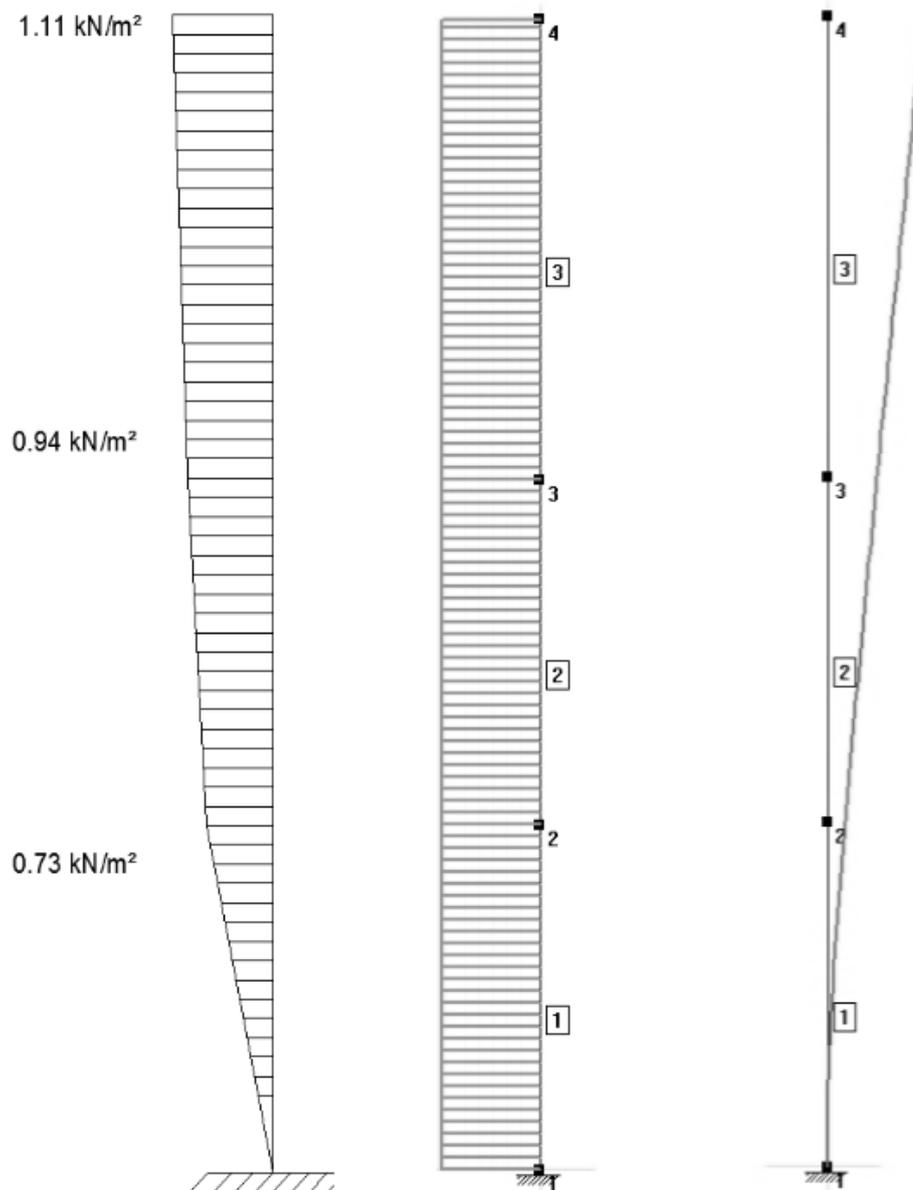
Figure 5.8: Non-uniform load, uniform load and displacement in Strusoft Frame Analysis.
