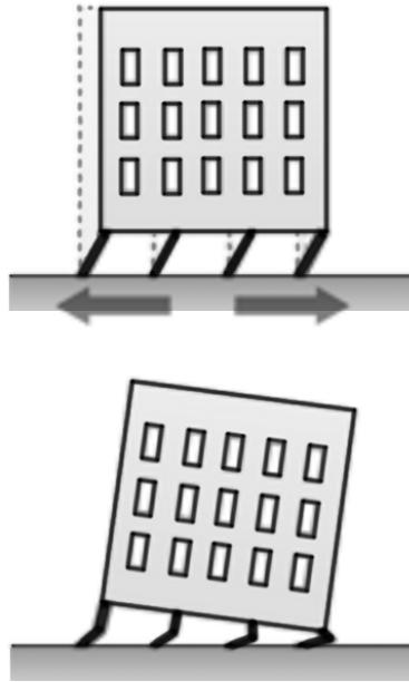
Figure 3.10: Illustration of a soft story collapse [56].
