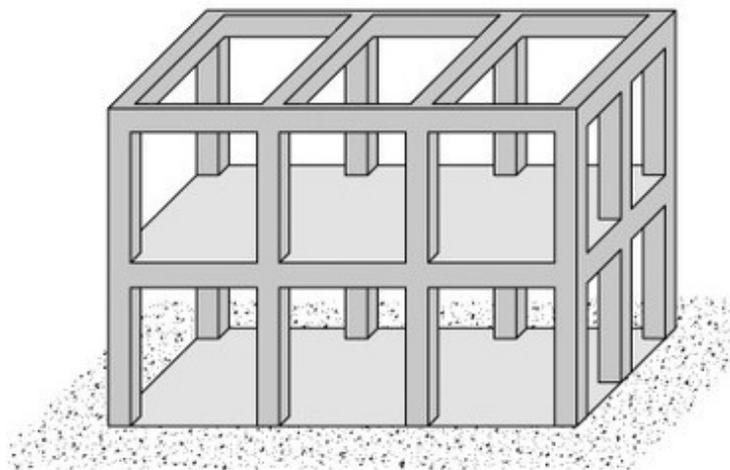
Figure 2.2: Illustration of a rigid frame [25].
