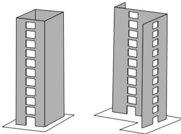
Figure 2.4: Illustration of coupled shear walls [64].
