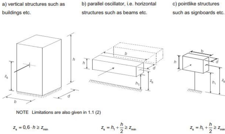
Figure 6.1 — General shapes of structures covered by the design procedure. The structural dimensions and the reference height used are also shown.
