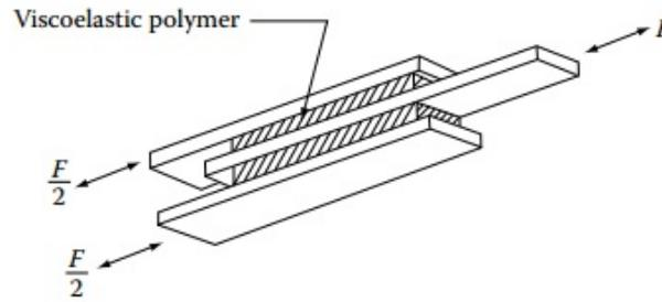
Figure 3.14: Illustration of viscoelastic damper [64].
