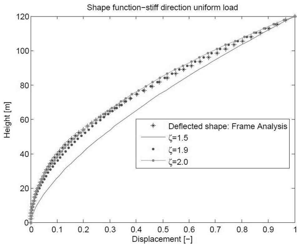
Figure 5.10: Shape function with uniform load in stiff direction.
