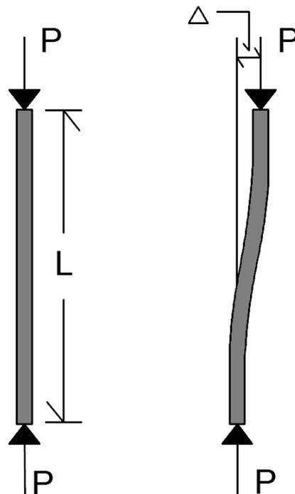
Figure 3.9: Illustration of P-delta effect [58].
