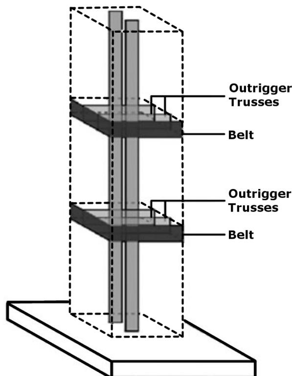
Figure 2.5: Illustration of an outrigger system [19].
