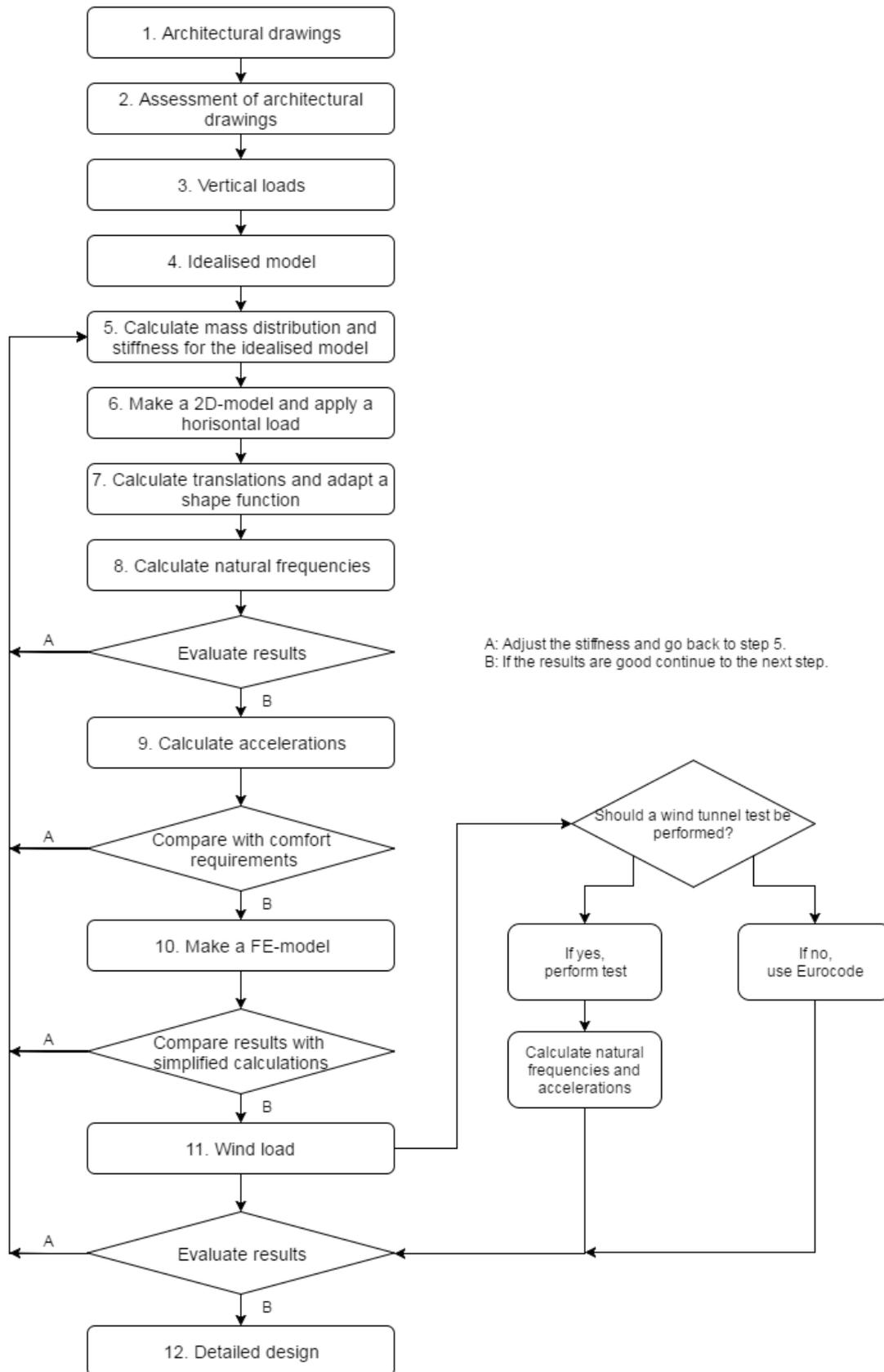
Figure 4.1: Calculation flowchart to follow when doing the preliminary design.
