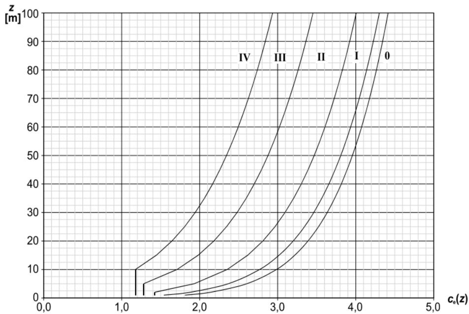
Figure 4.2 — Illustrations of the exposure factor  $c_e(z)$  for  $c_{e0}=1,0$ ,  $k_f=1,0$
