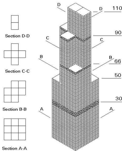
Figure 2.11: Illustration of a bundled tube system [55].
