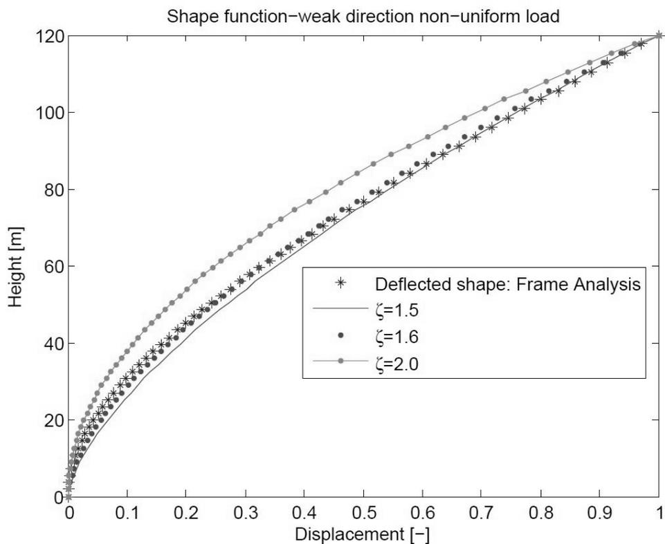
Figure 5.11: Shape function with non-uniform load in weak direction.
