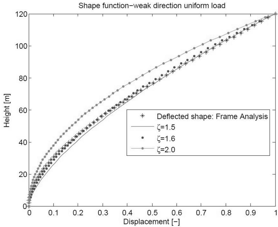
Figure 5.9: Shape function with uniform load in weak direction.
