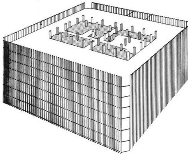
Figure 2.9: Illustration of tube system [26].
