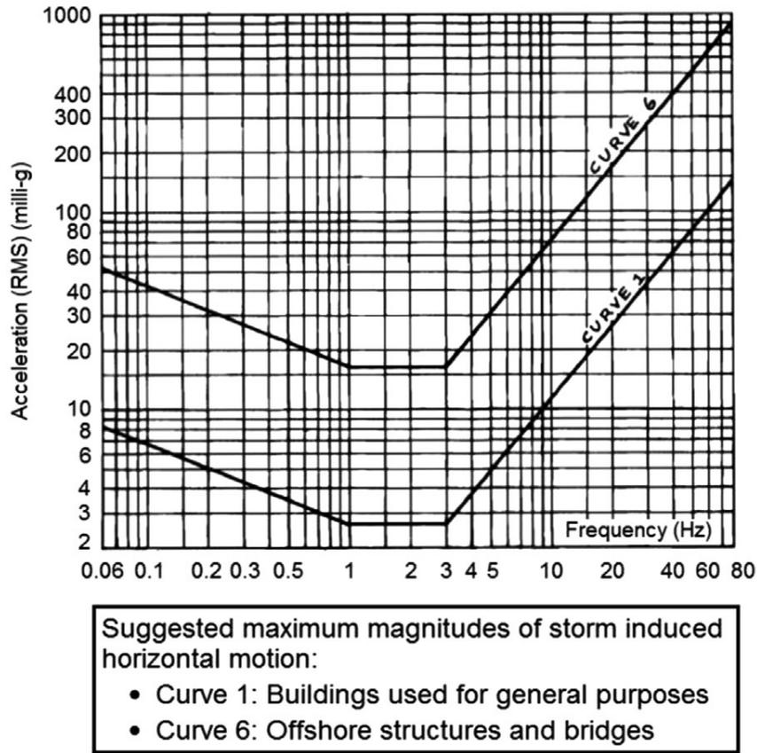
Figure 3.6: Suggested maximum rms acceleration by Irwin, later adopted into ISO 6897 [36].
