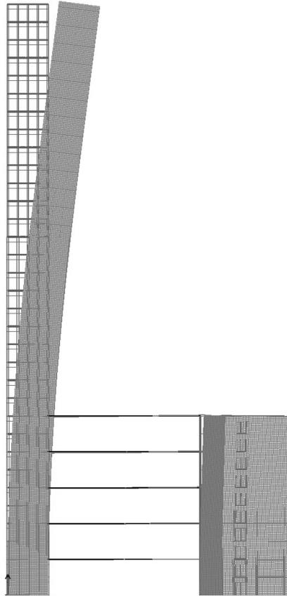
Figure 5.23: Illustration of the displacement of the coupled cores.
