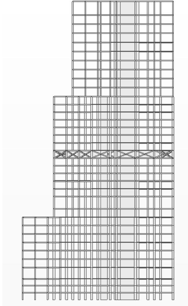
Figure 5.26: Illustration of building with outrigger.
