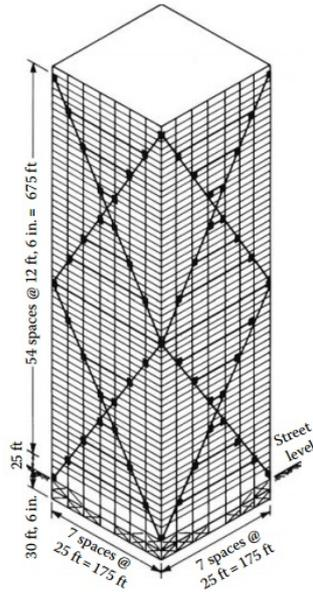
Figure 2.10: Illustration of an exterior diagonal tube system.
