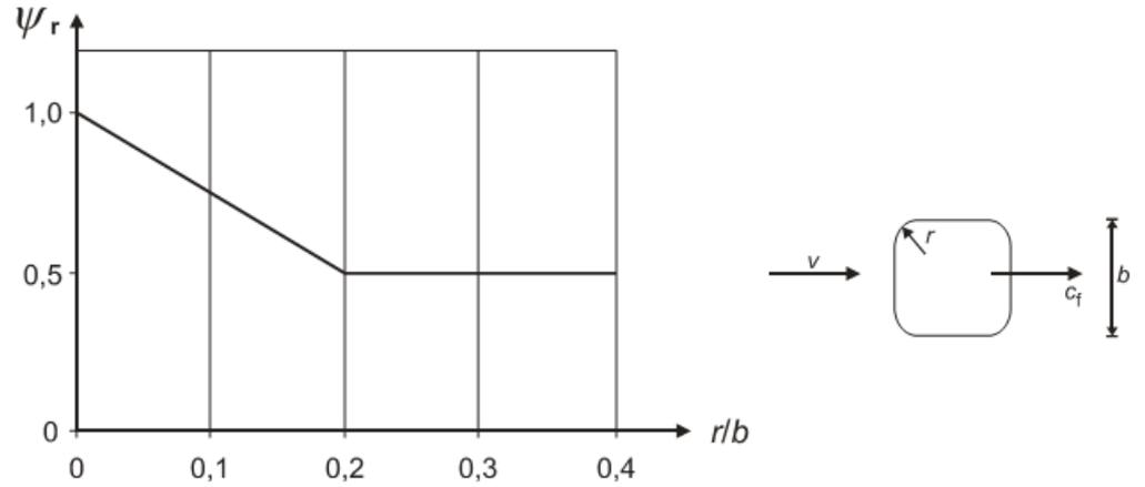
Figure 7.24 — Reduction factor  $\psi_r$  for a square cross-section with rounded corners
