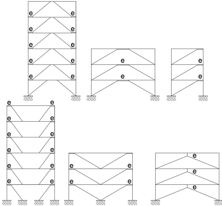
Figure 2.7: Illustration of eccentric braced frames [64].
