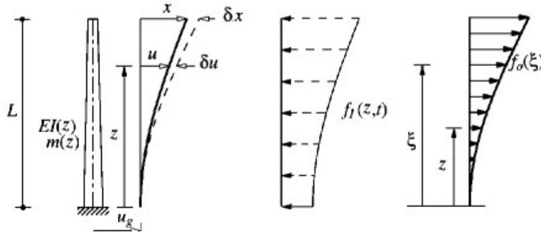
Figure 4.2: Displacement in building when subjected to a uniformly distributed load [10].
