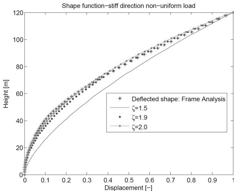
Figure 5.12: Shape function with non-uniform load in stiff direction.
