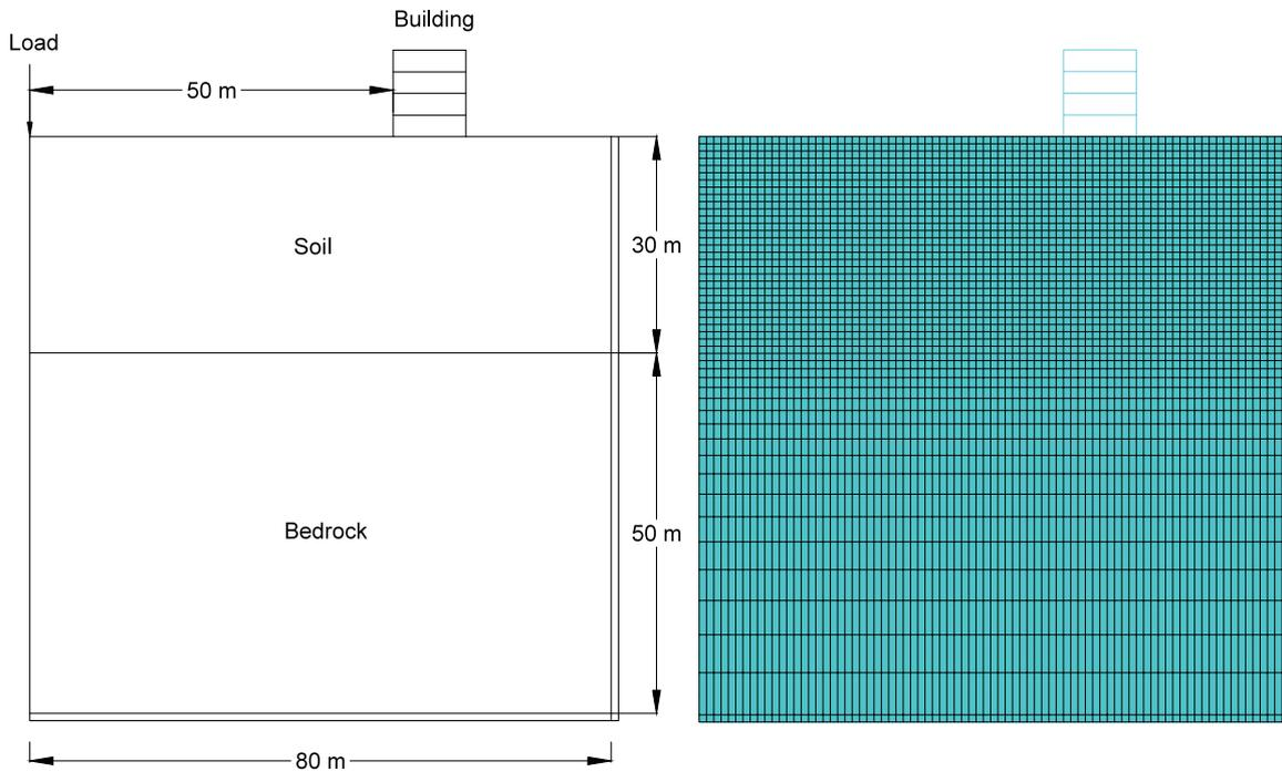
**Figure 5.8:** Soil model (left) and mesh (right)
