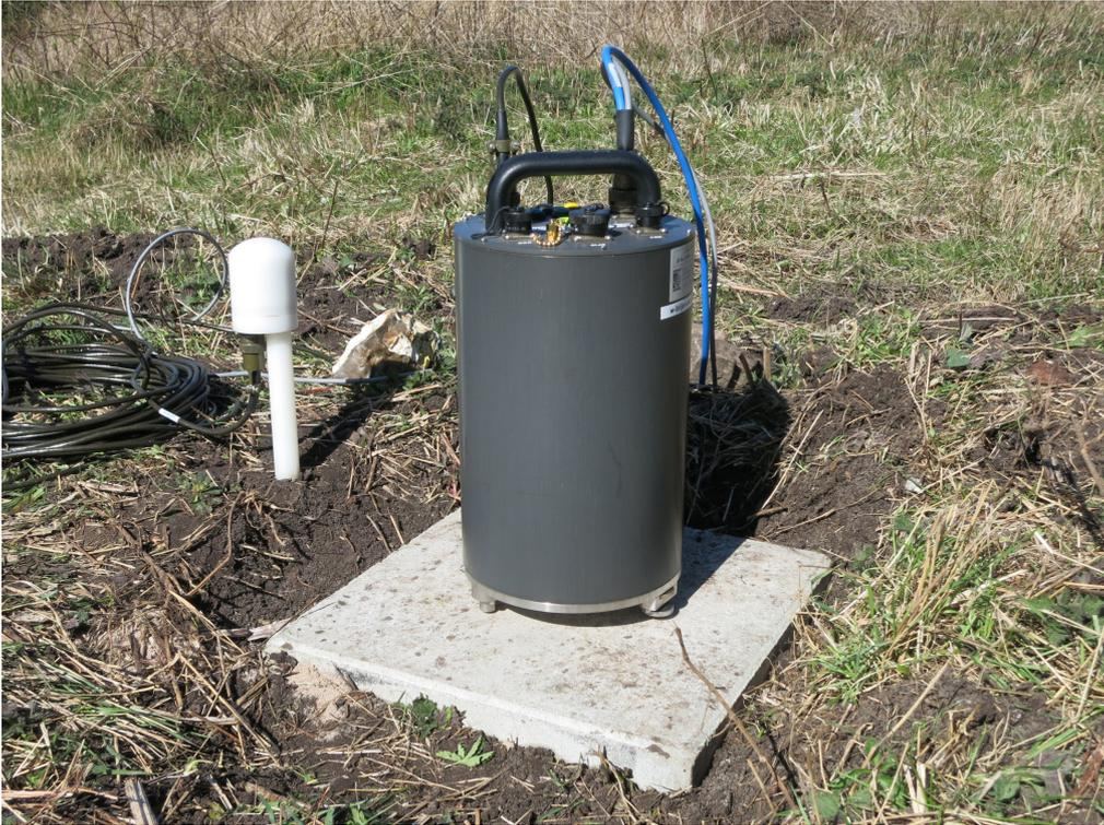
**Figure 4.4:** Photograph of the seismometer used in the measurements.
