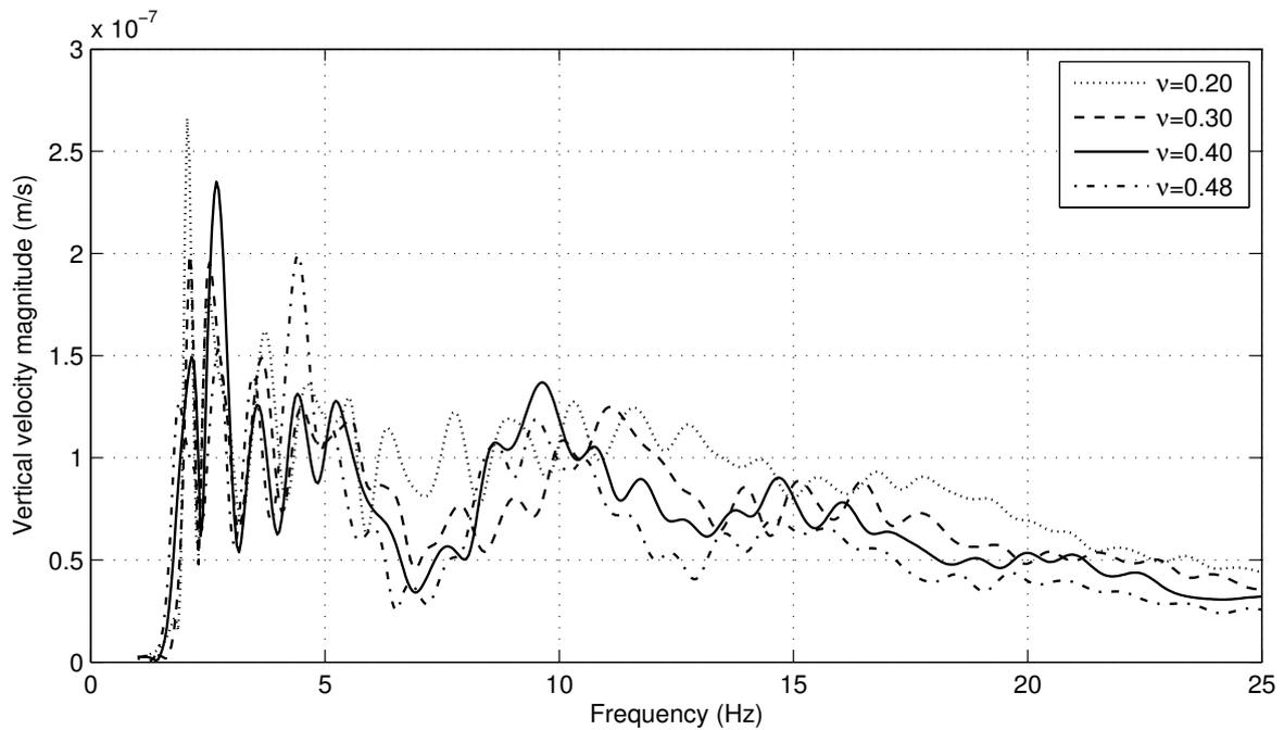
**Figure 5.4:** Effect of Poisson's ratio,  $\nu$ , on the vertical vibrations in the soil model.
