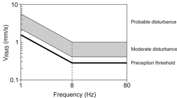
**Figure 2.9:** Vibration levels for perception threshold and disturbance. From [37].
