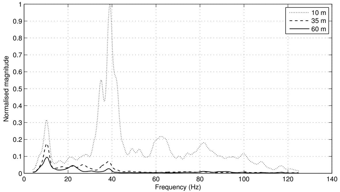
**Figure 4.13:** FFT by distance from track for a freight train. Normalised to the maximum amplitude.
