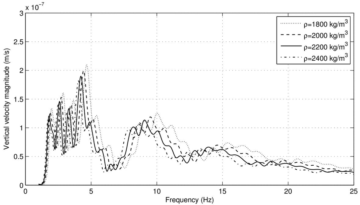
**Figure 5.3:** Effect of soil density,  $\rho$ , on the vertical vibrations in the soil model.
