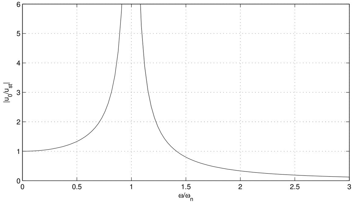
**Figure 3.2:** Displacement response for an undamped SDOF system under harmonic loading.
