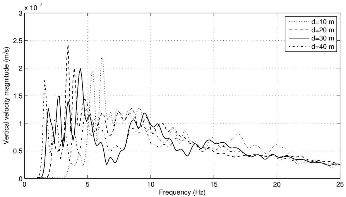
**Figure 5.6:** Effect of soil layer depth,  $d$ , on the vertical vibrations in the soil model.
