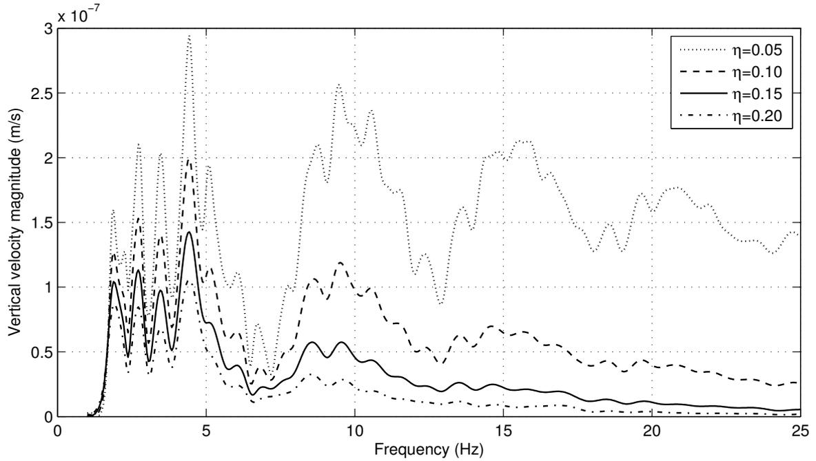
**Figure 5.5:** Effect of loss factor,  $\eta$ , on the vertical vibrations in the soil model.
