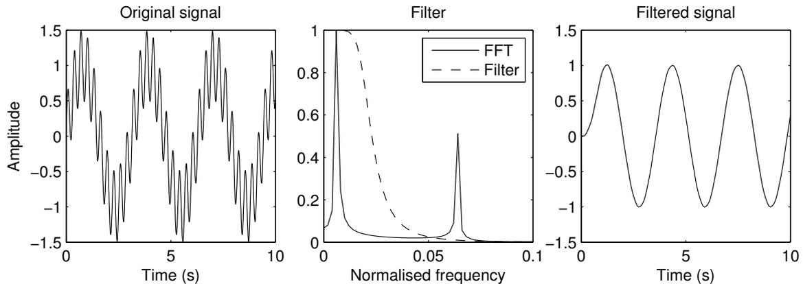
**Figure 4.3:** Original signal (left), low-pass filter applied (middle) and resulting filtered signal (right).
