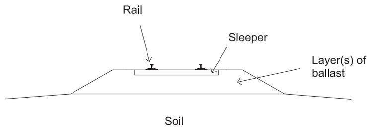
**Figure 2.6:** A schematic illustration of a typical railway track structure.
