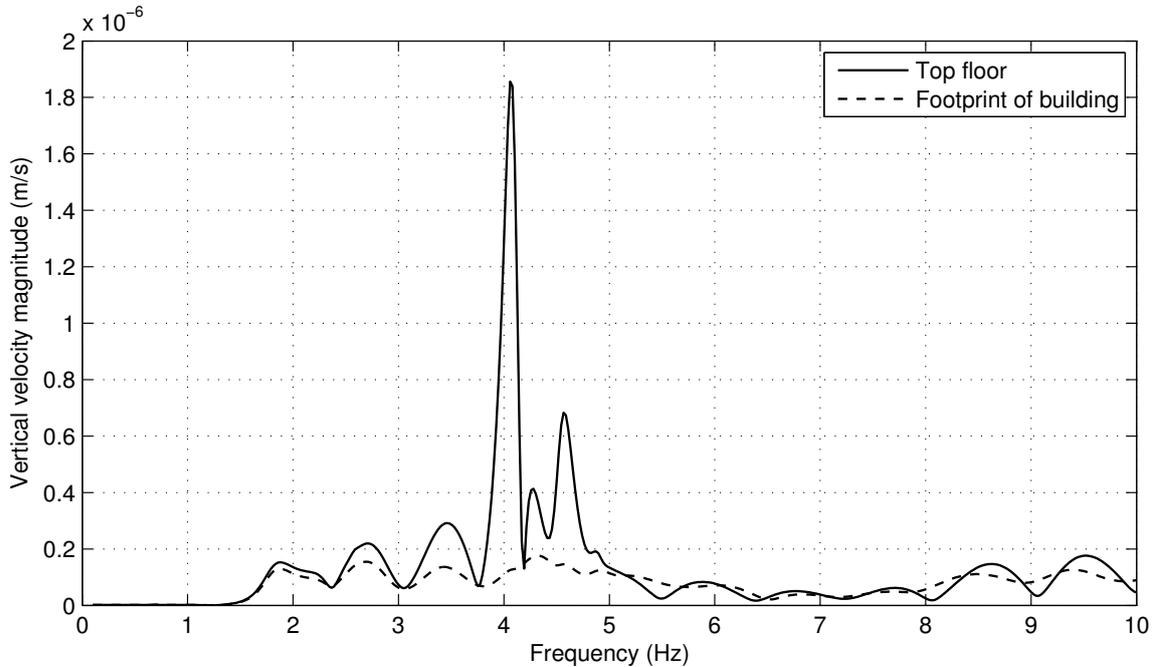
**Figure 5.9:** RMS velocities in nodes in the top floor of the building and at the footprint of the building.
