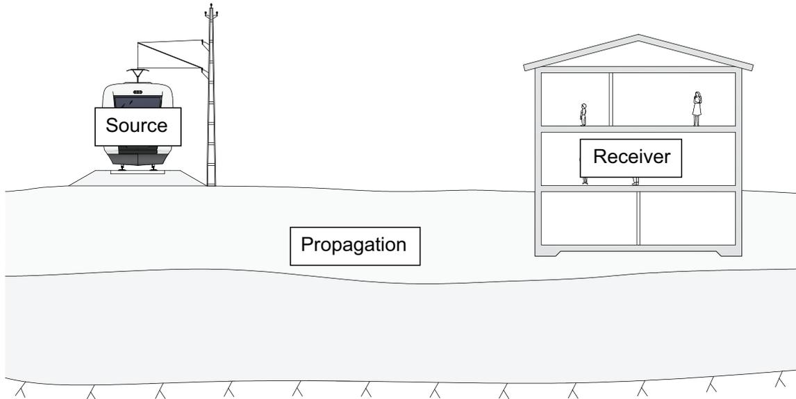
**Figure 2.5:** Transmission process for railway-induced ground vibrations.
