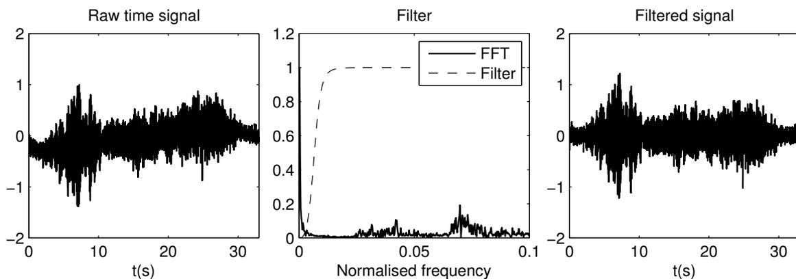
**Figure 4.8:** Example of a signal being filtered.
