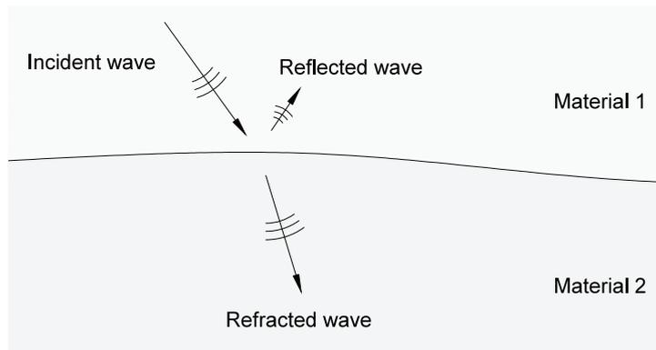
**Figure 2.4:** Reflection and refraction of a wave.
