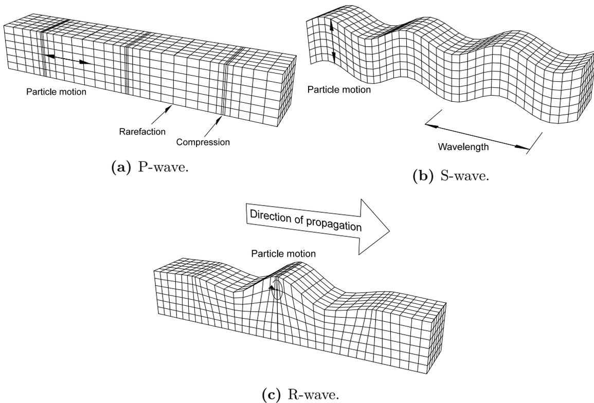
**Figure 2.2:** The three main wave types relevant to ground vibrations.
