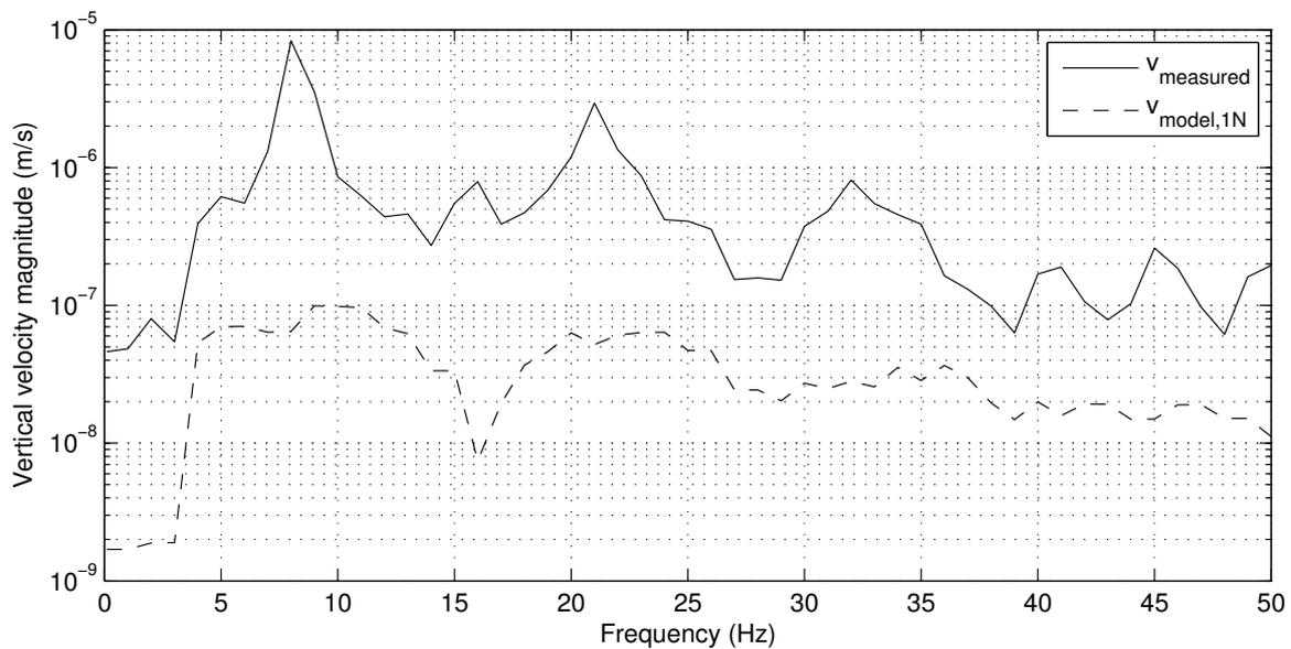
**Figure 5.11:** Measured response for a freight train and simulated response for a 1 N load at 60 m from track.
