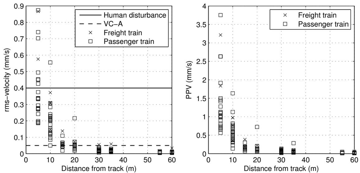
**Figure 4.11:** RMS values (left) and peak particle velocities (right) of vertical velocities for all trains as a function of distance from the track.
