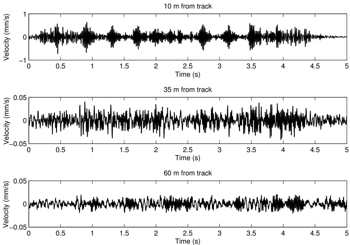
**Figure 4.9:** Velocity at different distances for a commuter train. Note that the y-axes are scaled differently.
