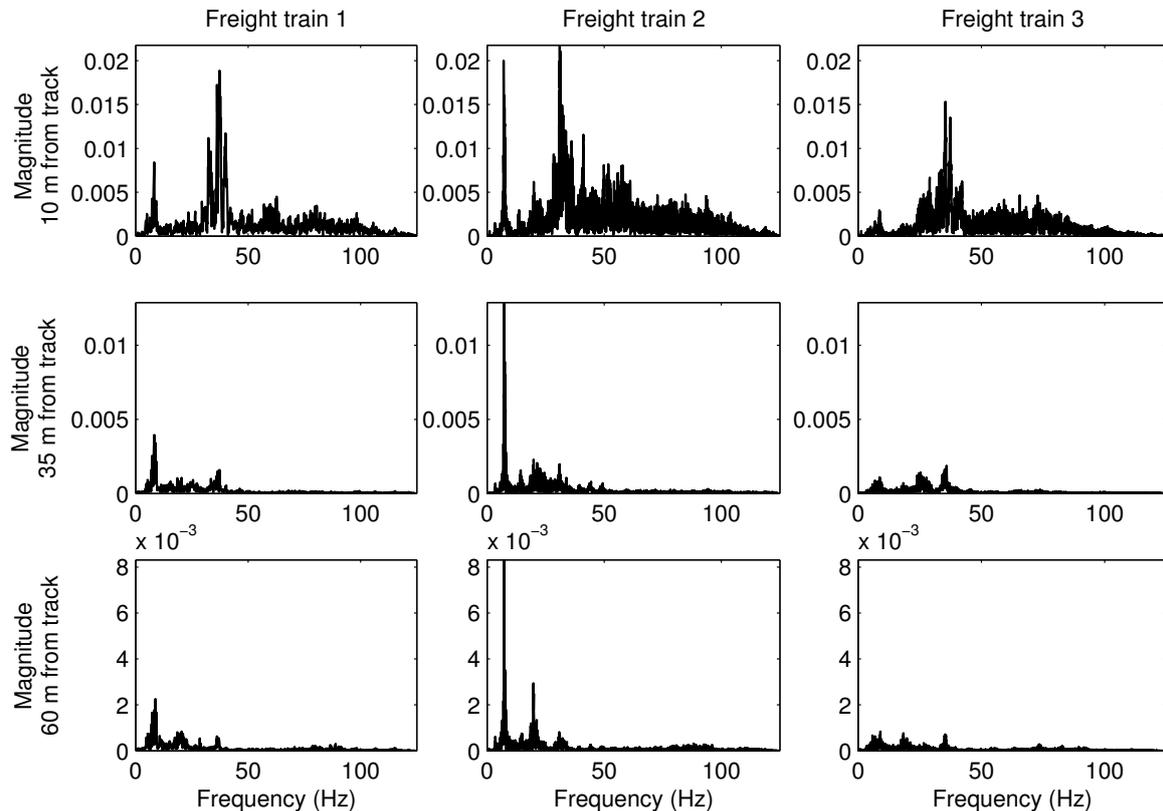
**Figure 4.12:** FFT for three different freight trains and distances from the track.
