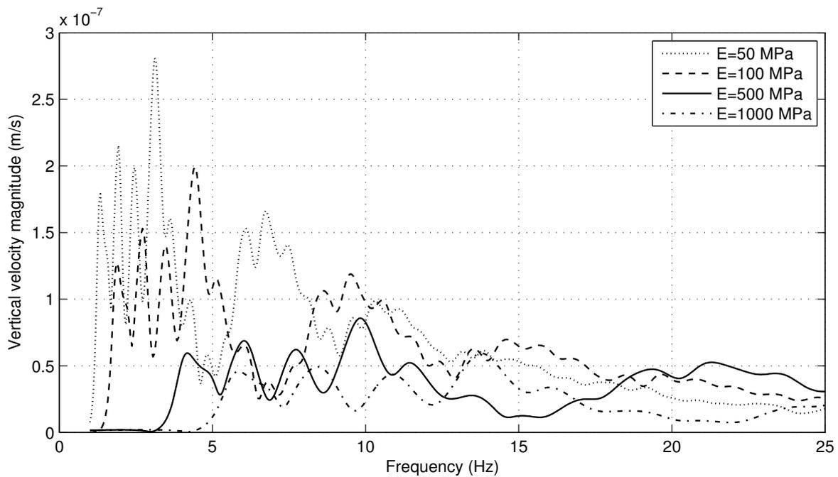
**Figure 5.2:** Effect of elastic modulus,  $E$ , on the vertical vibrations in the soil model.
