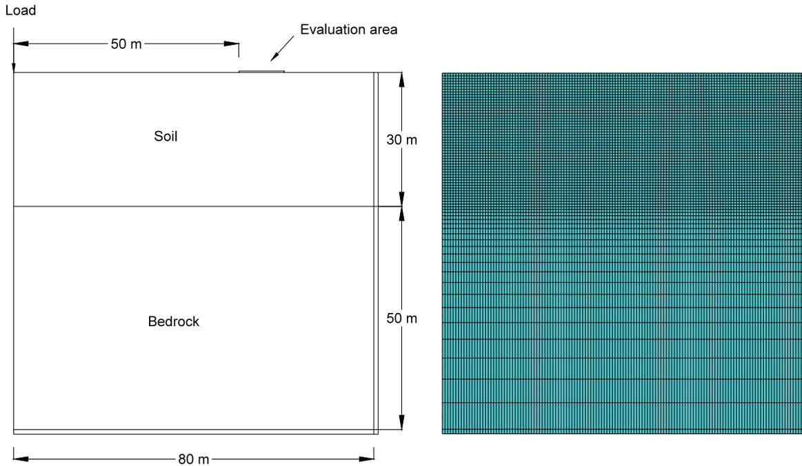
**Figure 5.1:** Soil model (left) and mesh (right).
