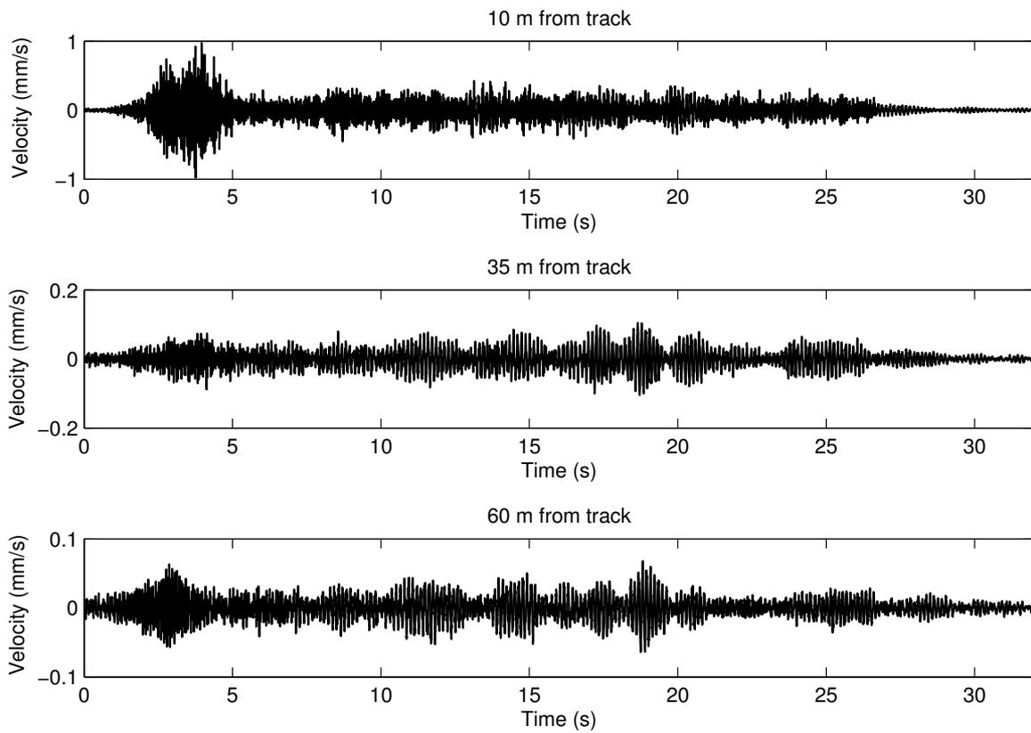
**Figure 4.10:** Velocity at different distances for a freight train. Note that the y-axes are scaled differently.
