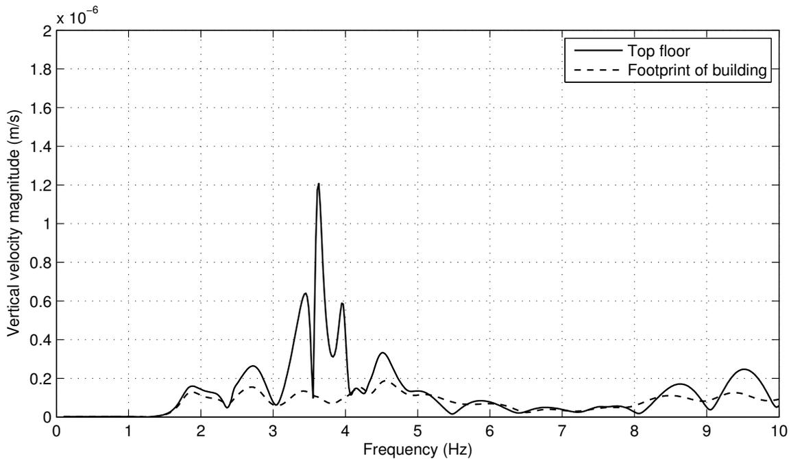
**Figure 5.10:** RMS velocities in nodes in the top floor of the building and at the footprint of the building when the eigenfrequency of the top floor has been lowered.
