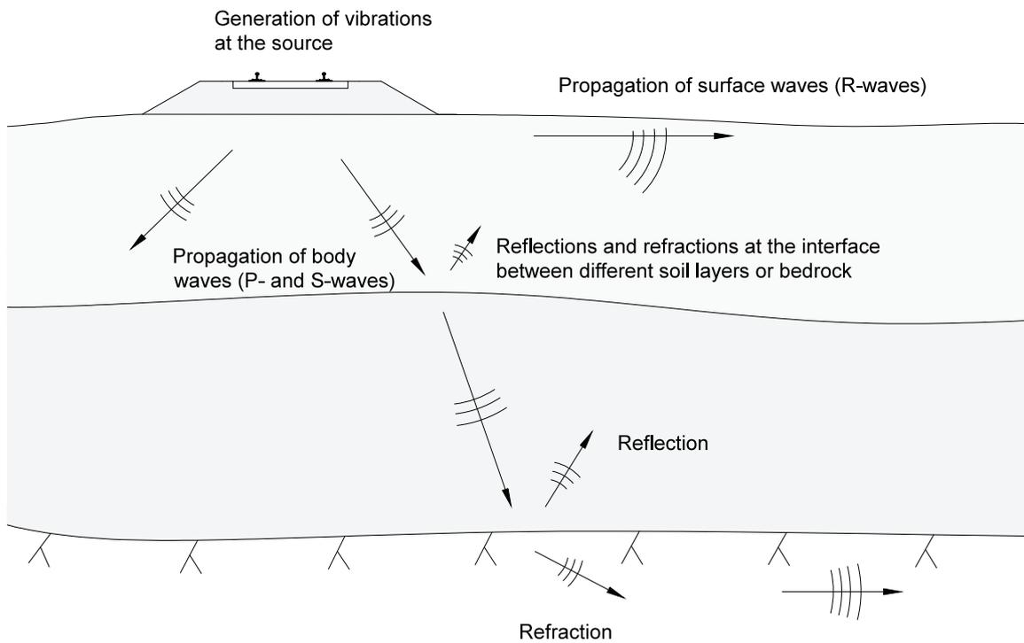
**Figure 2.8:** Illustration of the propagation process for ground vibrations.
