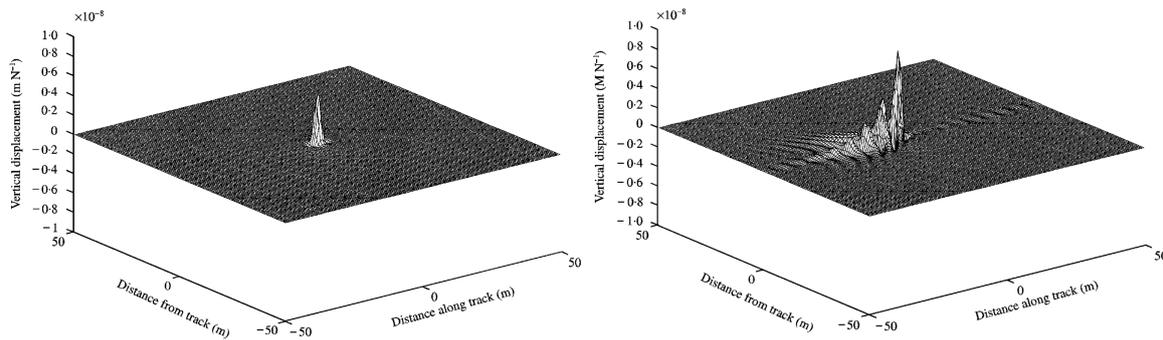
**Figure 2.7:** Vertical displacements in the soil for a concentrated force moving at a speed below the R-wave speed (left) and above the R-wave speed (right). From [42].
