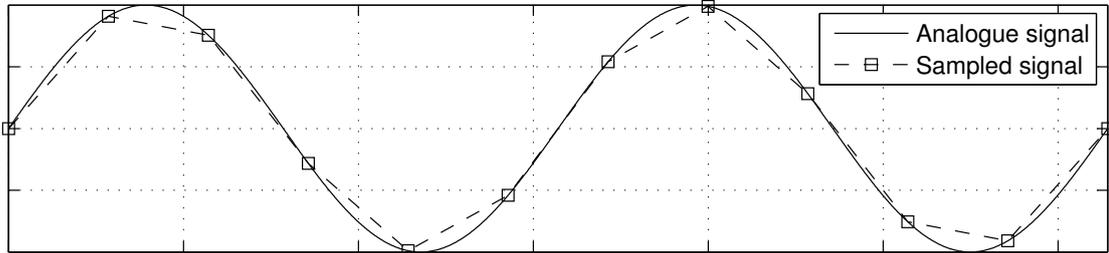
**Figure 4.1:** Analogue and sampled signal.
