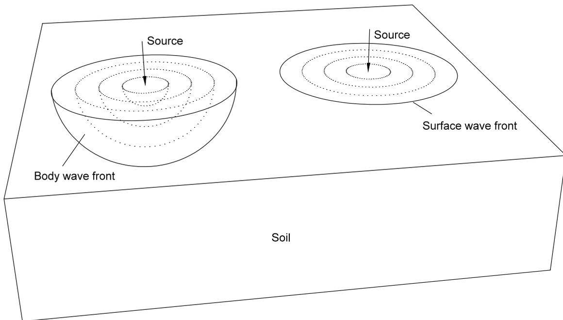
**Figure 2.3:** Geometrical attenuation for body waves (left) and surface waves (right).
