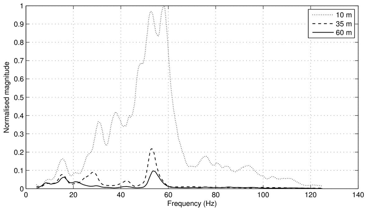
**Figure 4.14:** FFT by distance from track for a commuter train. Normalised to the maximum amplitude.
