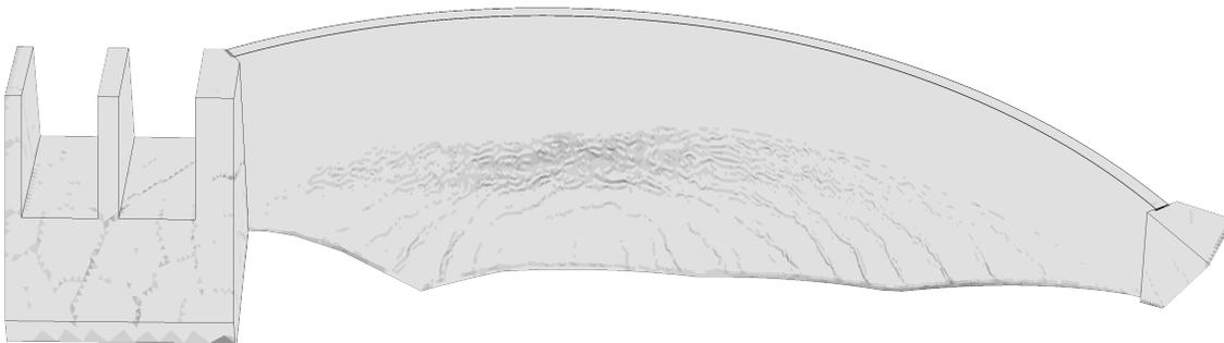
Figure 7.55: Crack propagation in January the second year on the downstream surface.
