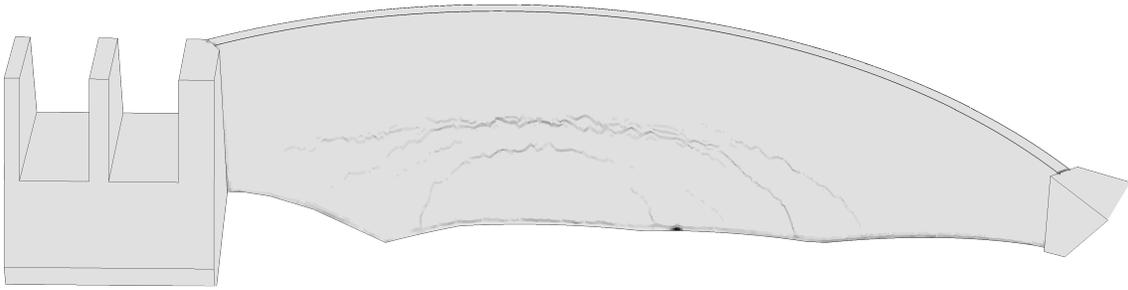
Figure 7.35: Crack propagation due to gravity and hydrostatic pressure alone on the downstream surface.
