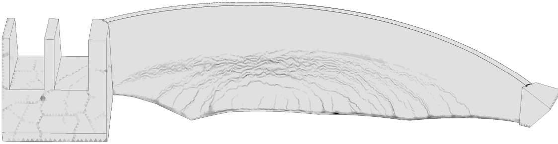
Figure 7.39: Crack propagation in January the second year on the downstream surface.
