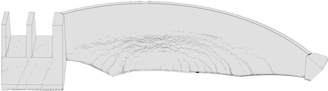
Figure 7.44: Crack propagation in January the first year on the downstream surface.
