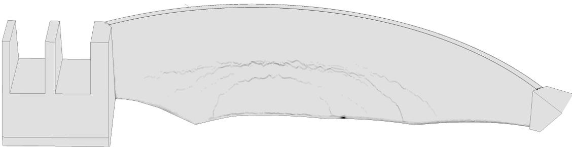
Figure 7.36: Crack propagation in July the first year on the downstream surface.
