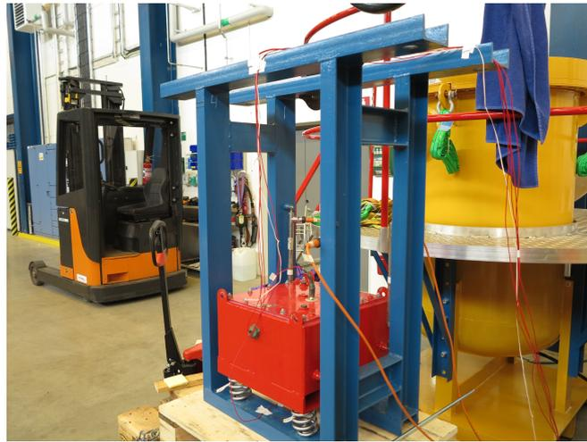
Figure 3.3: Here the box is mounted on the frame with the tank in the background and wires connected to the measuring devices.
