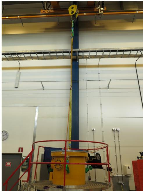
Figure 3.6: The traverse crane at the top of the picture is connected to the submerged box via a set of crane slings
