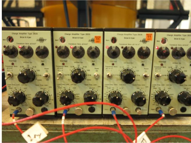
Figure 3.9: The charge amplifiers used by both the accelerometers and the pressure gauges were connected to the data acquisition unit.
