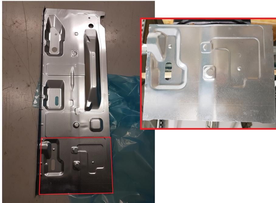
Figure 1.2: Photographs of the full size floor panel and the cut-out from the panel.
