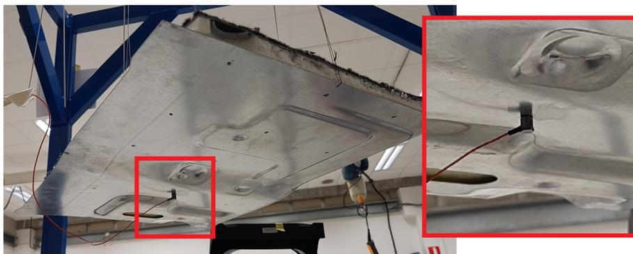
Figure 4.11: Panel and carpet with accelerometer.
