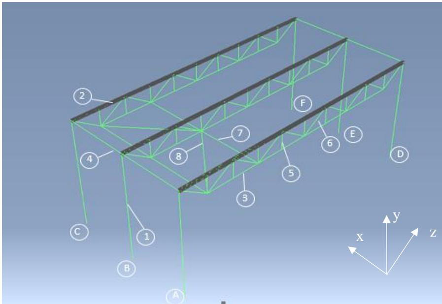
Figure 14. An overview of the warehouse, without its roof, in Abaqus with all its parts numbered.
