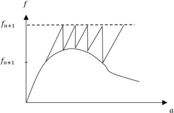
Figure 33. Displaying an softening response after peak load. When the load  $f_{(n+1)}$  is held constant, the equilibrium equations would continue forever since the softening branch would not be traced correctly. Adapted from (Ottosen & Ristinmaa, 2005).
