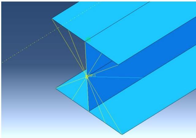
Figure 18. The point RP-1, acts as an master node. The yellow strings are an illustration of the slave nodes connection to the master.
