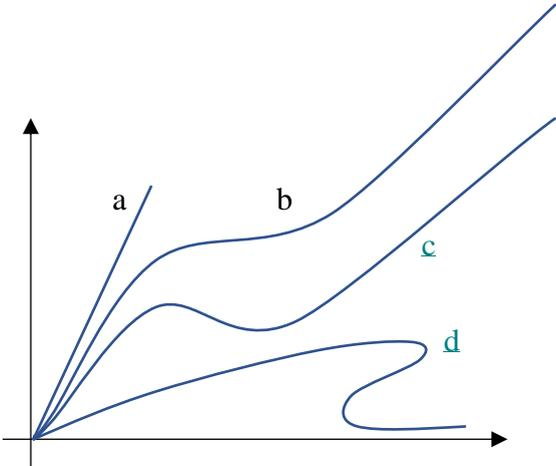
Figure 32. showing the different force-displacement behaviors a, linear b, nonlinear(monotonic increase) c, nonlinear (with local minimum) and d, general nonlinear behavior including snap-back.
