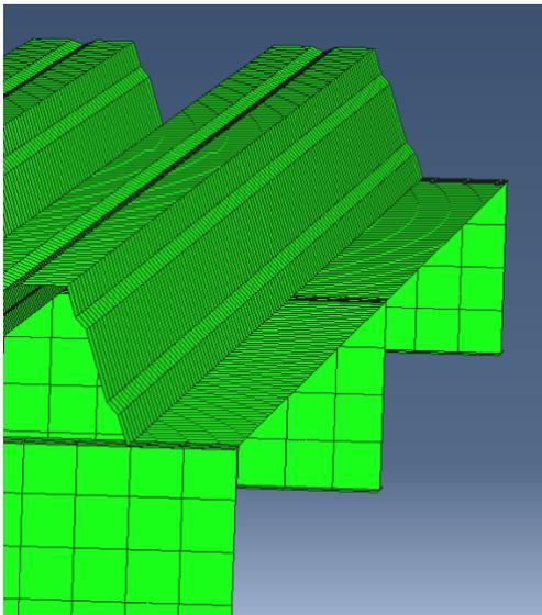
Figure 29. the outer flange which needed to be made thicker to obtain converged solutions.
