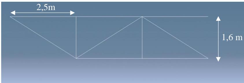
Figure 5. A detailed view of the truss.
