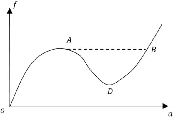
Figure 35. If the arc-length method wouldn't be used in this case the information after point A would be lost. Adapted from (Ottosen & Ristinmaa, 2005).
