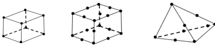
Figure 10. Composition of different types of nodal elements adapted from (Sharcnet, u.d.).
