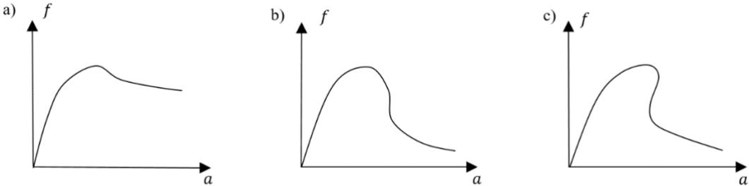
Figure 34. a, Ductile response. b, Brittle response. c, The snap-back phenomenon. Adapted from (Ottosen & Ristinmaa, 2005).
