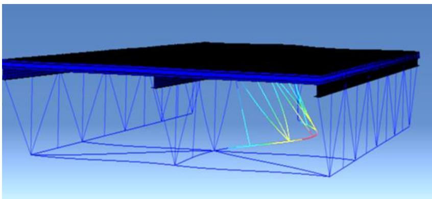
Figure 31. The buckling of the bottom-chord.
