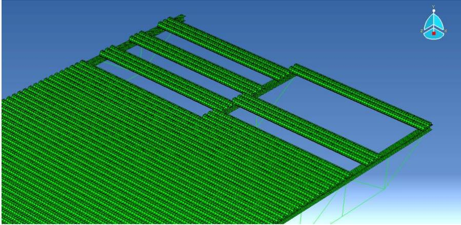
Figure 20. An illustration of how the CGI-plates are connected in model A.
