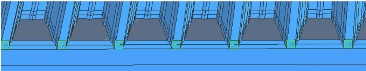
Figure 23. Spot-weld fastener with a distance of 0,280 m.
