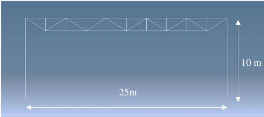
Figure 4. Section AA of fig.3, showing the truss and columns.
