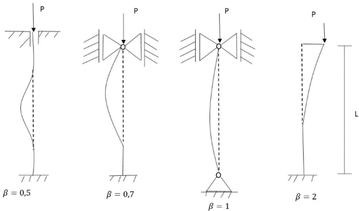
Figure 11. Euler's four different buckling cases where the value of  $\beta$  is based on the attachment of the bar. Adapted from (Pettersson, 1971).
