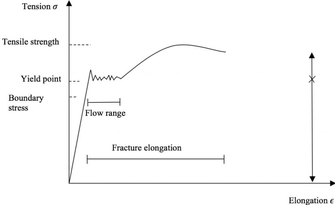
Figure 7. A typical stress/strain diagram for steel. Adapted from (Hanses, 2015).
