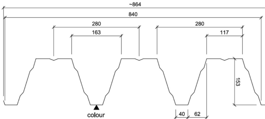
Figure 8. A typical profile used for CGI plates. Note that the distances changes between different profiles. From appendix A, Rukki technical drawing.
