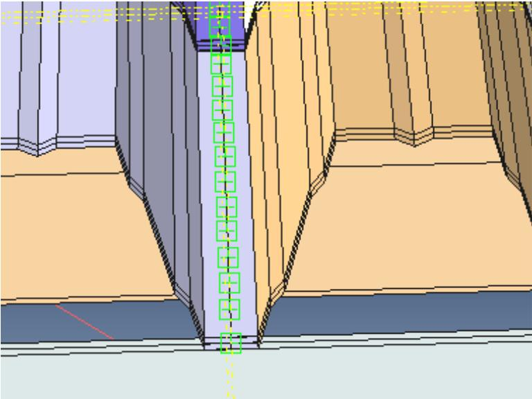
Figure 24. Fasteners used to connect the CGI-plates to each other in model A.
