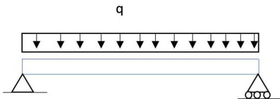
Figure 12. The load case used as for the static analysis.
