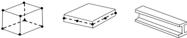
Figure 9. Different element types adapted from (Sharcnet, u.d.).
