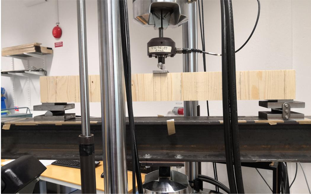
**Figure B.3:** Test setup for in-plane loaded Specimen 2 beam.
