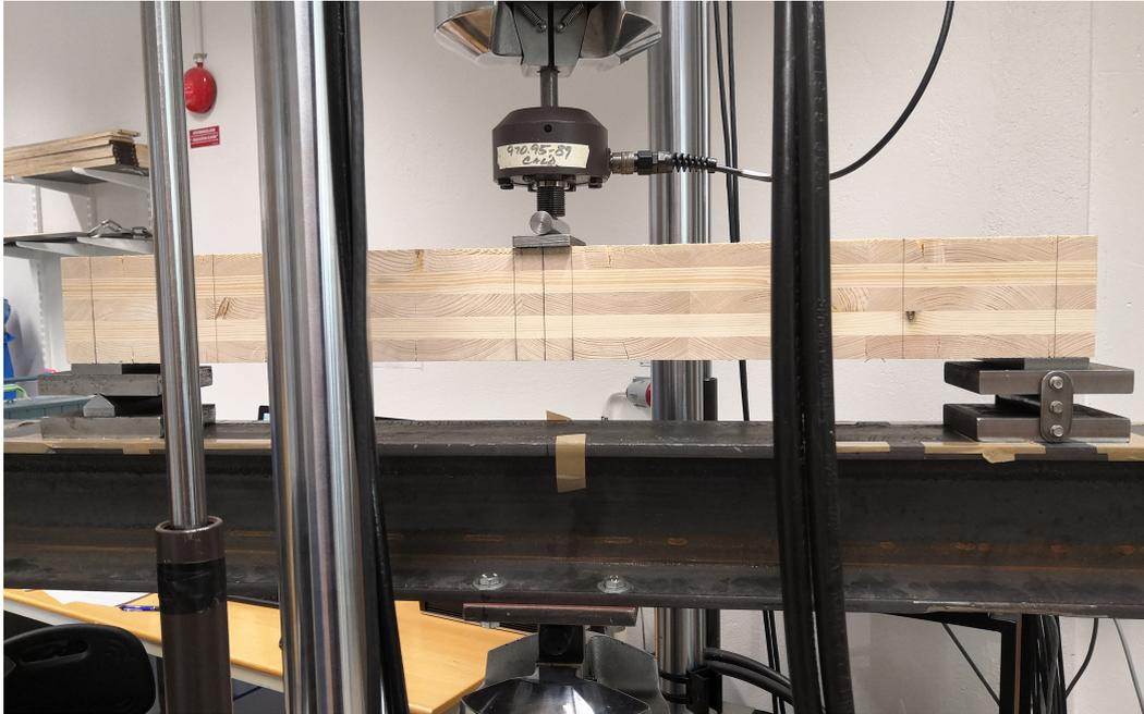
**Figure B.4:** Test setup for out-of-plane loaded Specimen 2 beam.
