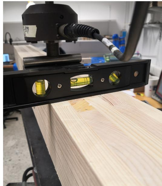
(b) Example of slope of a CLT-beam.
