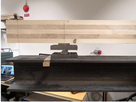
(a) Fix support with a steel plate mounted on top.
