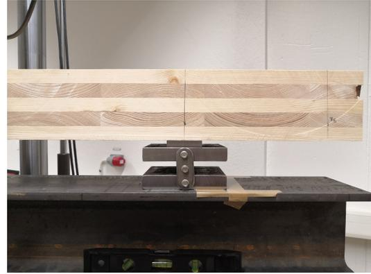
(b) Roller support with a steel plate mounted on top.
